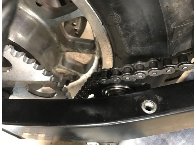
Figure 28: Chain tensioner guiding chain over swingarm. Photo Source: Craig Stephens
