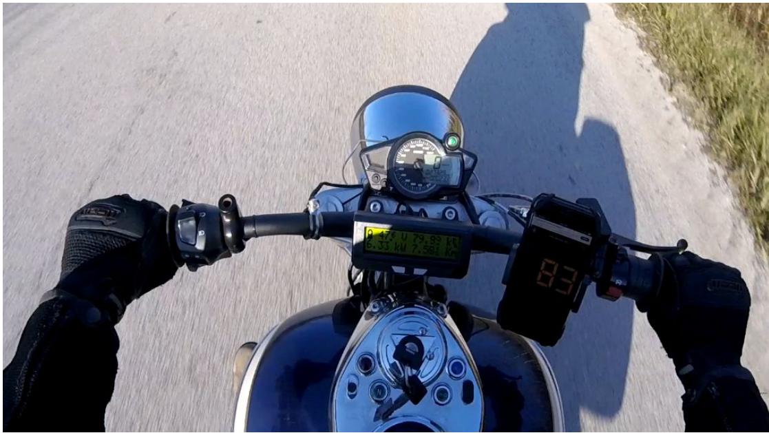
Figure 36: Cycle Analyst shows 79.99km/h while GPS reads 83km/h. Photo Source: Craig Stephens
