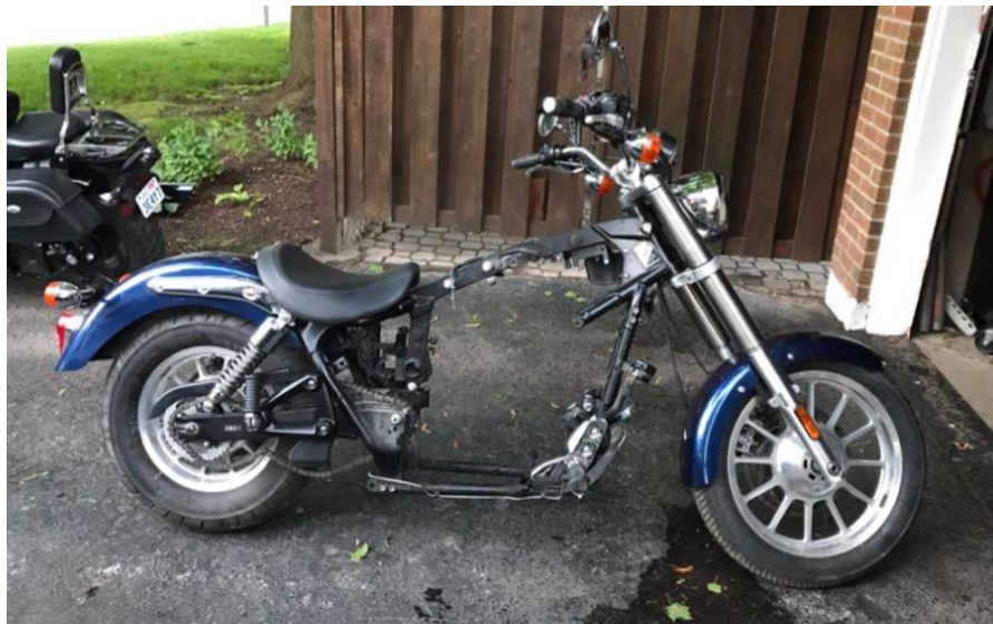
Figure 2: 2010 Triumph America rolling chassis. Photo Source: Craig Stephens
