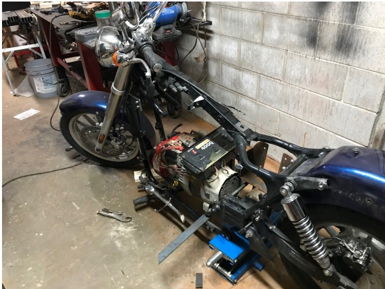
Figure 8: Generator mounting. Photo Source: Craig Stephens
