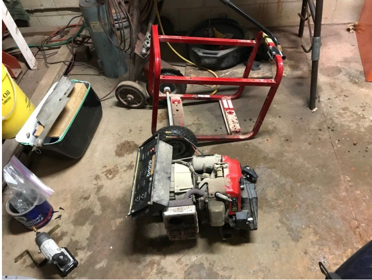
Figure 7: Generac generator disassembly. Photo Source: Craig Stephens
