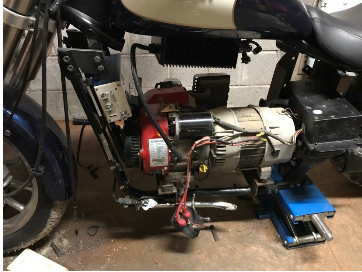
Figure 16: Controller mounted up front (blue and white) Photo Source: Craig Stephens
