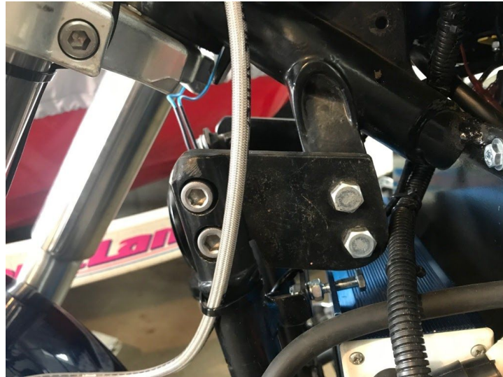
Figure 6: Manufactured hanger brackets increasing length by 3 inches. Photo Source: Craig Stephens
