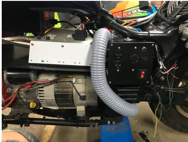
Figure 23, 24 & 25: 12V fan mounted on the underside of the bike and 2" corrugated tubing directing air into the motor. Photo Source: Craig Stephens
