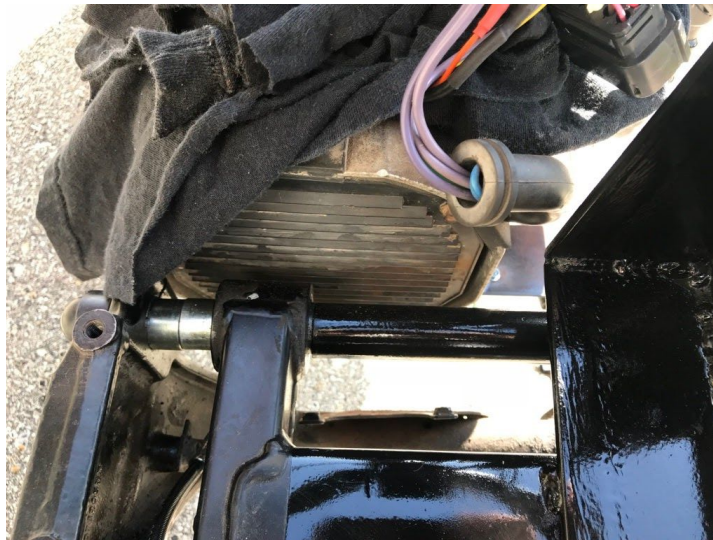
Figure 22: Jackshaft modified with appropriate sleeving. Photo Source: Craig Stephens
