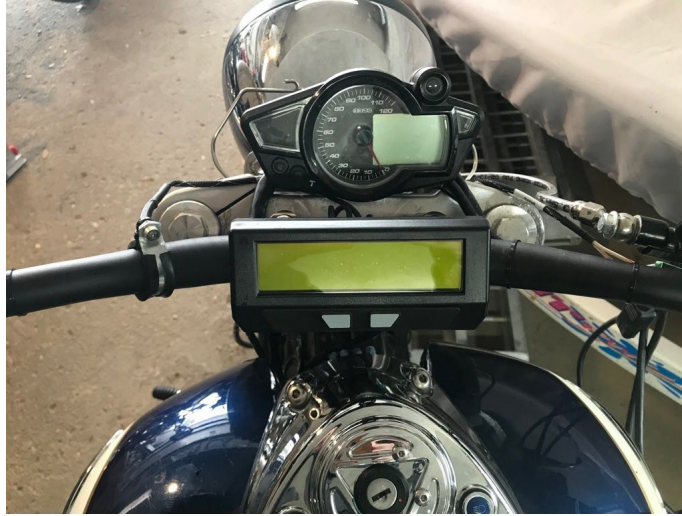
Figure 29: Cycle Analyst mounted. Photo Source: Craig Stephens
