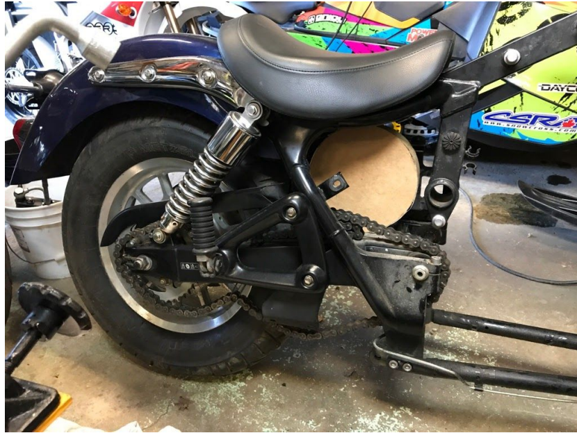
Figure 3: Motor mock-up. Photo Source: Craig Stephens
