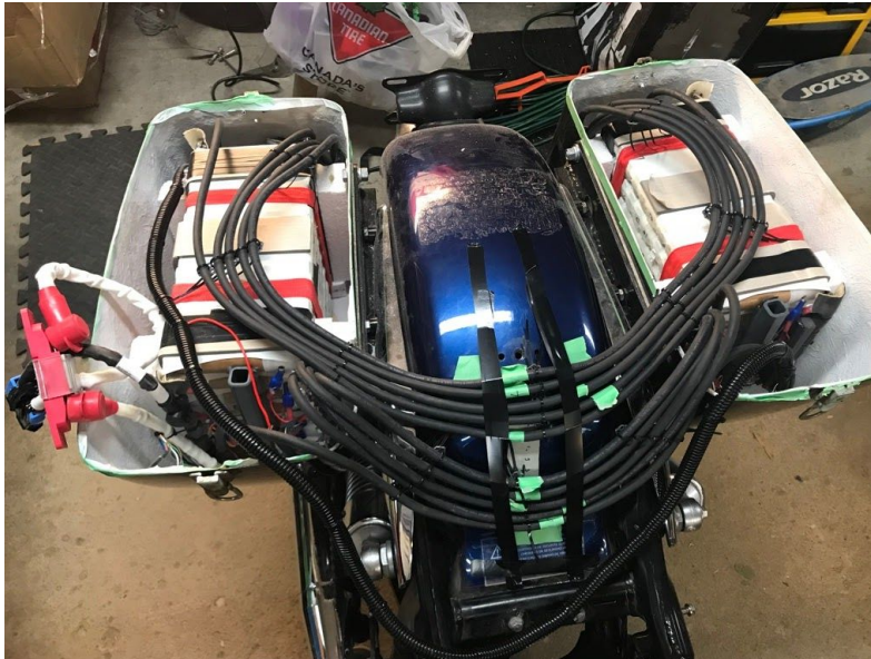
Figure 13: 11 Jumper cables connected between the batteries. Photo Source: Craig Stephens
