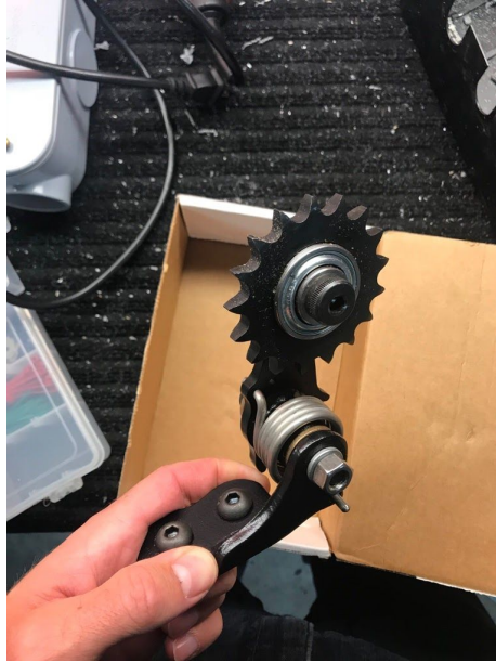
Figure 26: Chain tensioner. Photo Source: Craig Stephens
