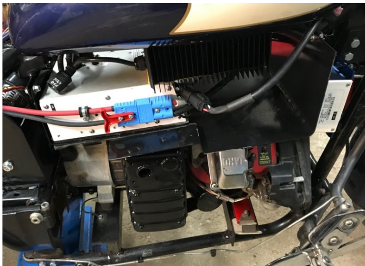
Figure 18: Quick connect handle mounted for safe battery cutoff. Photo Source: Craig Stephens
