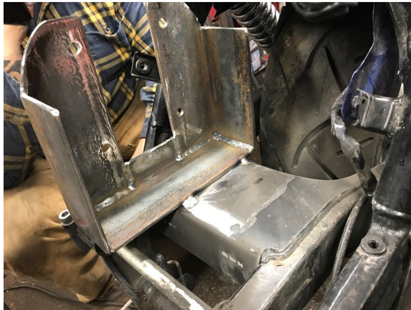
Figure 4: Motor mount built and installed. Photo Source: Craig Stephens
