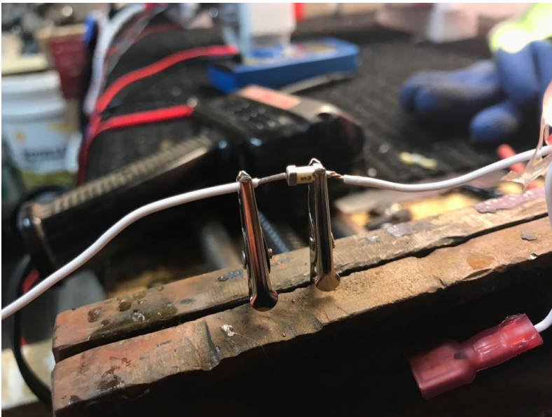
Figure 14: 4A micro fuses being soldered. Photo Source: Craig Stephens
