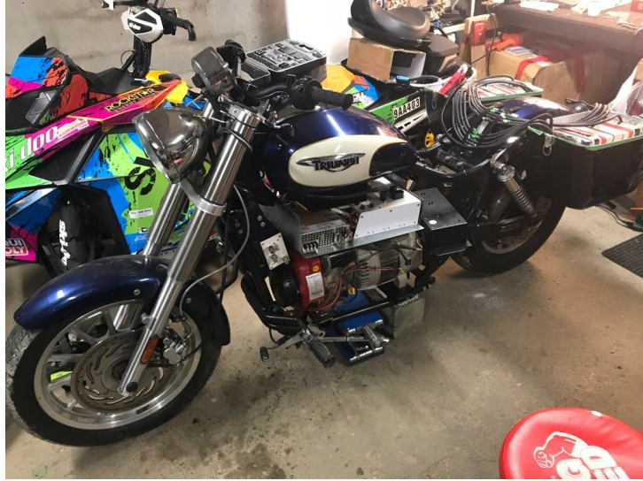
Figure 17: Fabricated tray holds the electronics box (white) and Meanwell RSP 3000 (silver). Photo Source: Craig Stephens
