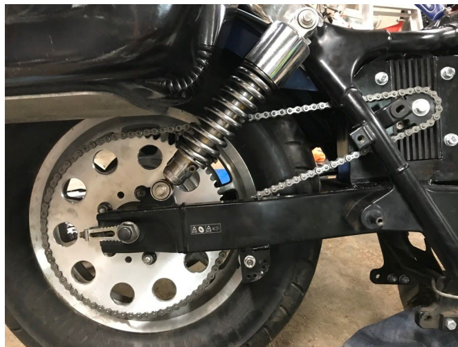
Figure 27: Chain tensioner installed. Photo Source: Craig Stephens
