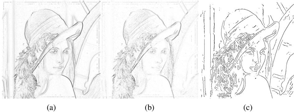
Figure 2.9: An example of local scale control. (a) Map of minimum reliable scale for gradient estimation. (b) Map of minimum reliable scale for second derivative estimation. (c) Detected edges. Six scales were used (0.5,1,2,4,8,16) and the shade of grey indicates the smallest scale at which gradient estimates are reliable. Black indicates scale at 0.5 pixel, lighter shades indicates higher scales, and white indicates that no reliable estimates could be made.
