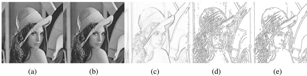
Figure 2.8: Canny edge detector process. (a) Original image. (b) Smoothed with Gaussian filter. (c) Map of intensity gradient. (d) Non-maximum suppressed "thin" version of edge map. (e) Edge map after hysteresis threshold.
