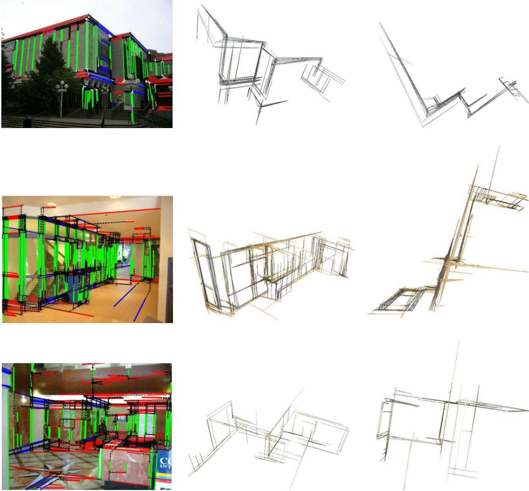
Figure 2.17: Line reconstruction results. The first column shows the Manhattan lines overlaying the original images. The second and third columns show perspective 3D views of the 3D line structures. Figure taken from [130].
