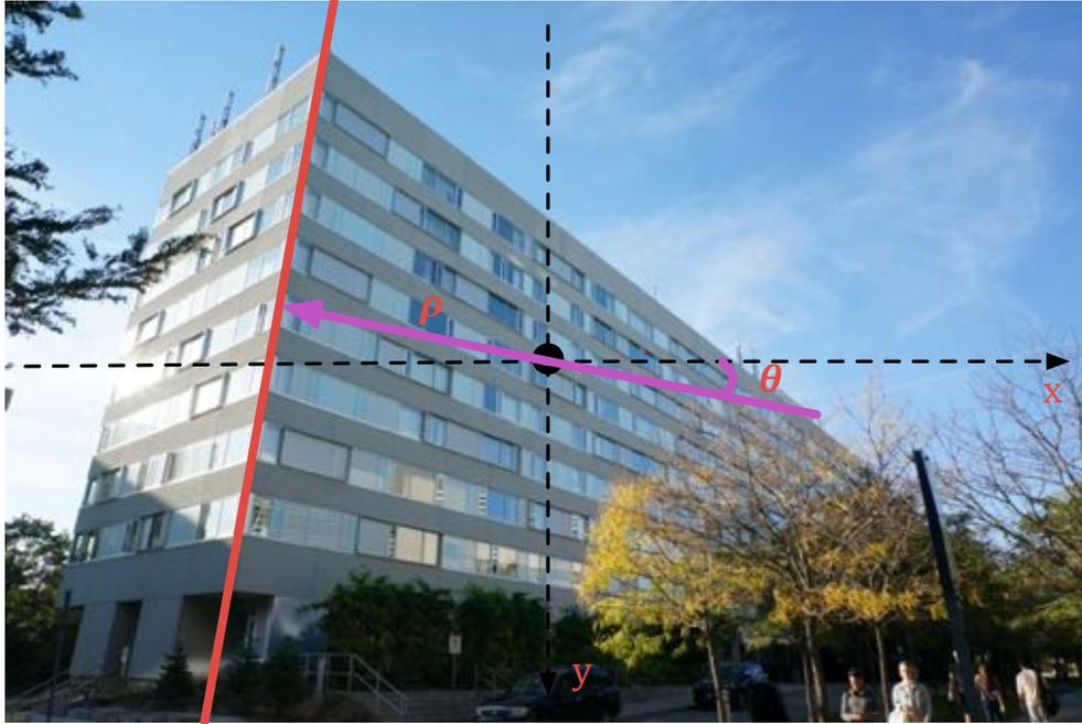
Figure 2.11: Hough parameters of a line.
