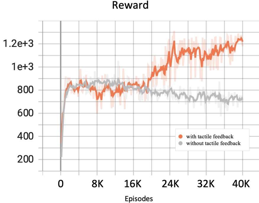
Figure 4.9: Accumulative moving average of rewards over the training episodes for both tactile-sensing and non-tactile agents. The tactile-based agent exploits contact feedback to more accurately adjust its pose, leading to a higher overall performance and faster convergence.
