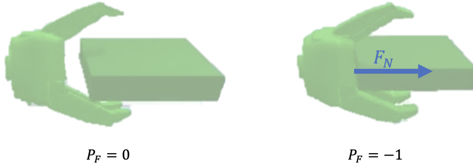
Figure 4.5: Graphical representation of the contact penalty term P_F . The penalty is applied when any contact force is detected by the gripper’s tactile sensors, thereby discouraging excessive force during pre-grasp.
