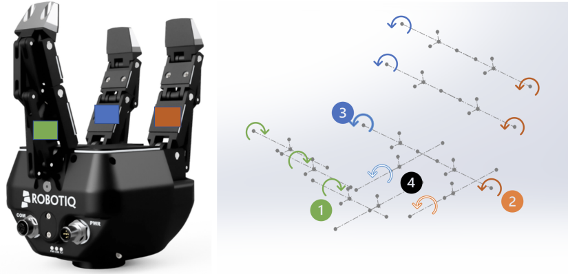
Figure 5.4: Robotiq 3F gripper with independently actuated proximal finger joints and mechanical linkages for the distal joints.
