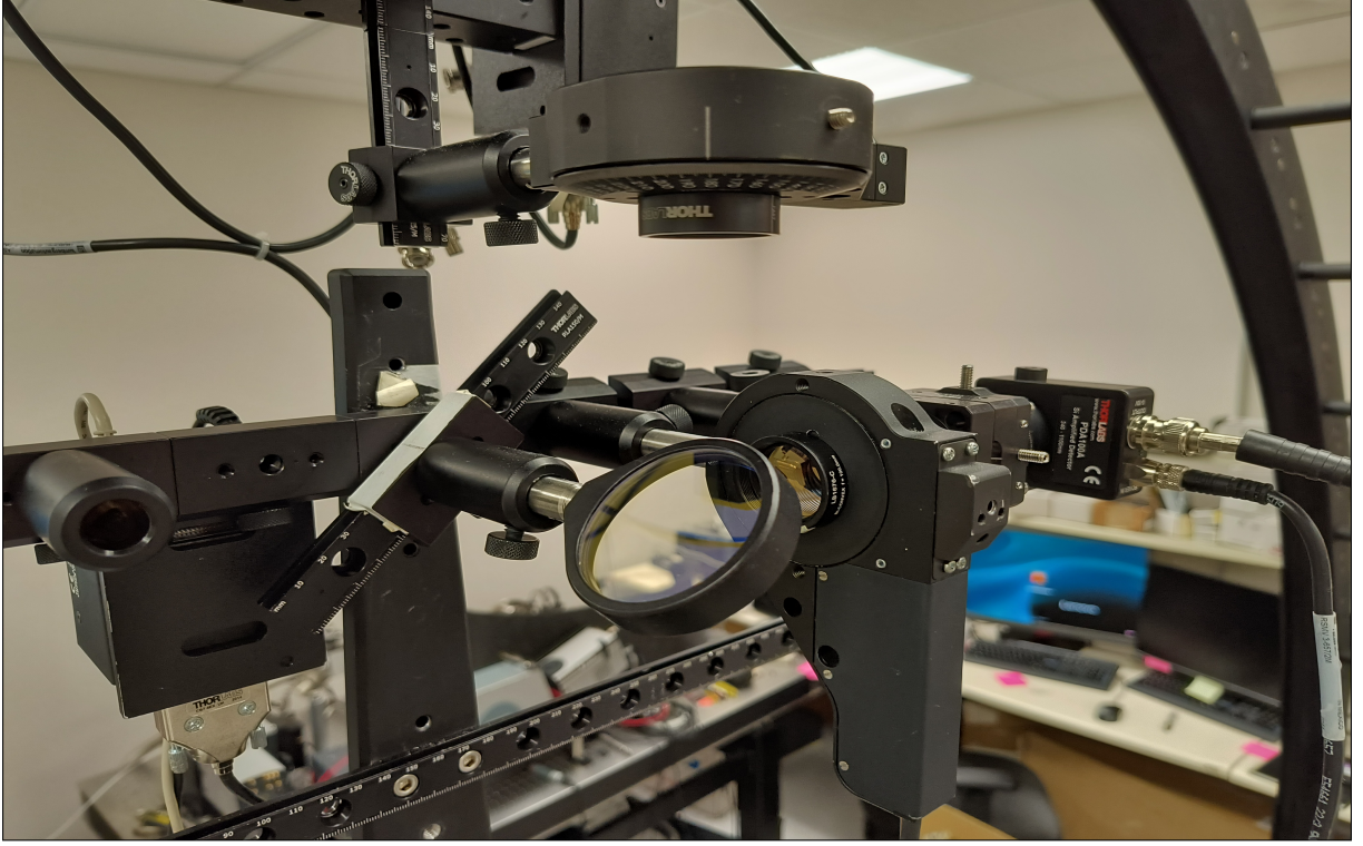
Figure 5.3: Beam splitter (BS) mounted on a 45^\circ rail to enable 0 - 5^\circ phase angle measurements without any setup restrictions
