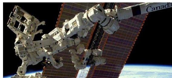
Fig. 43 Dextre robotic arm in operation on ISS. 157
