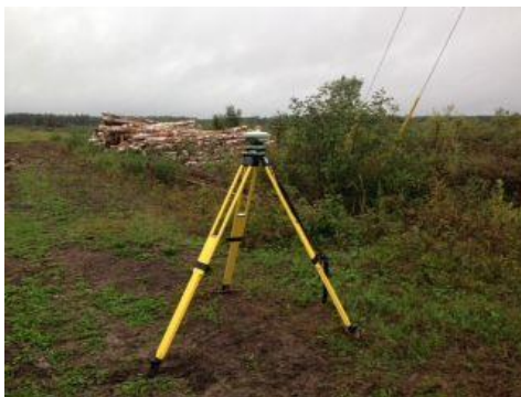
Figure 5.4: GPS base station for acquiring coordinates of plots
