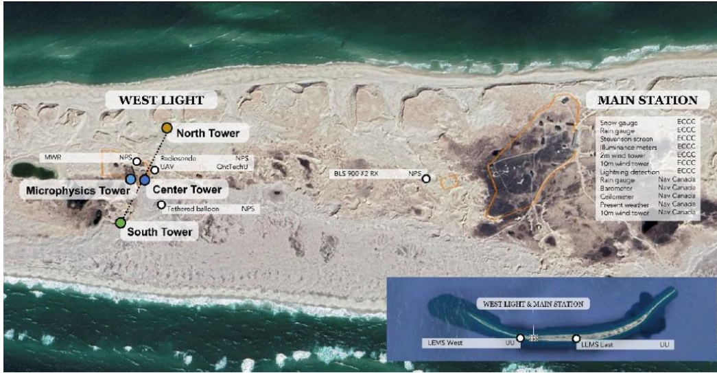
Figure 3.2 Sable Island instrument deployment during the campaign (from Fernando et al., 2025).
