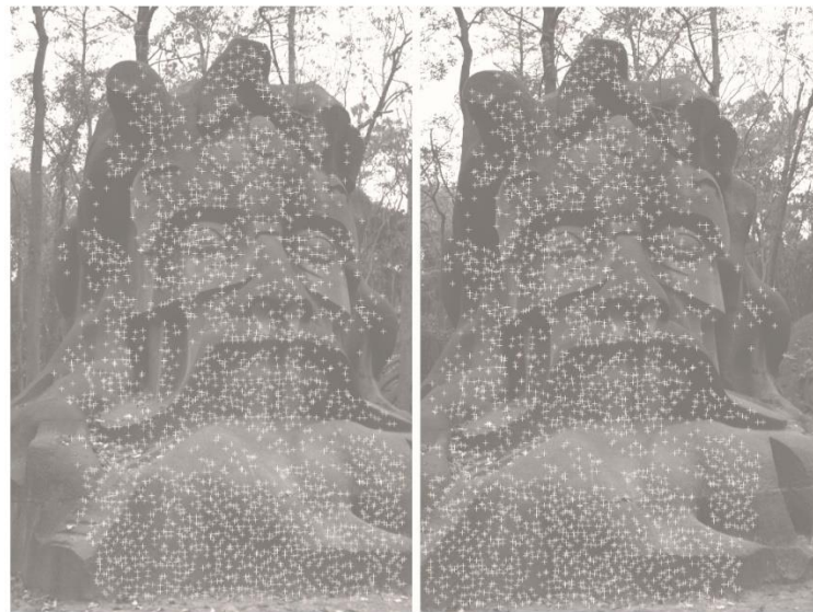
Figure 2.1: Dense tie point cloud from an image pair of a stone statue. Source: Zheng et al. (2013)
