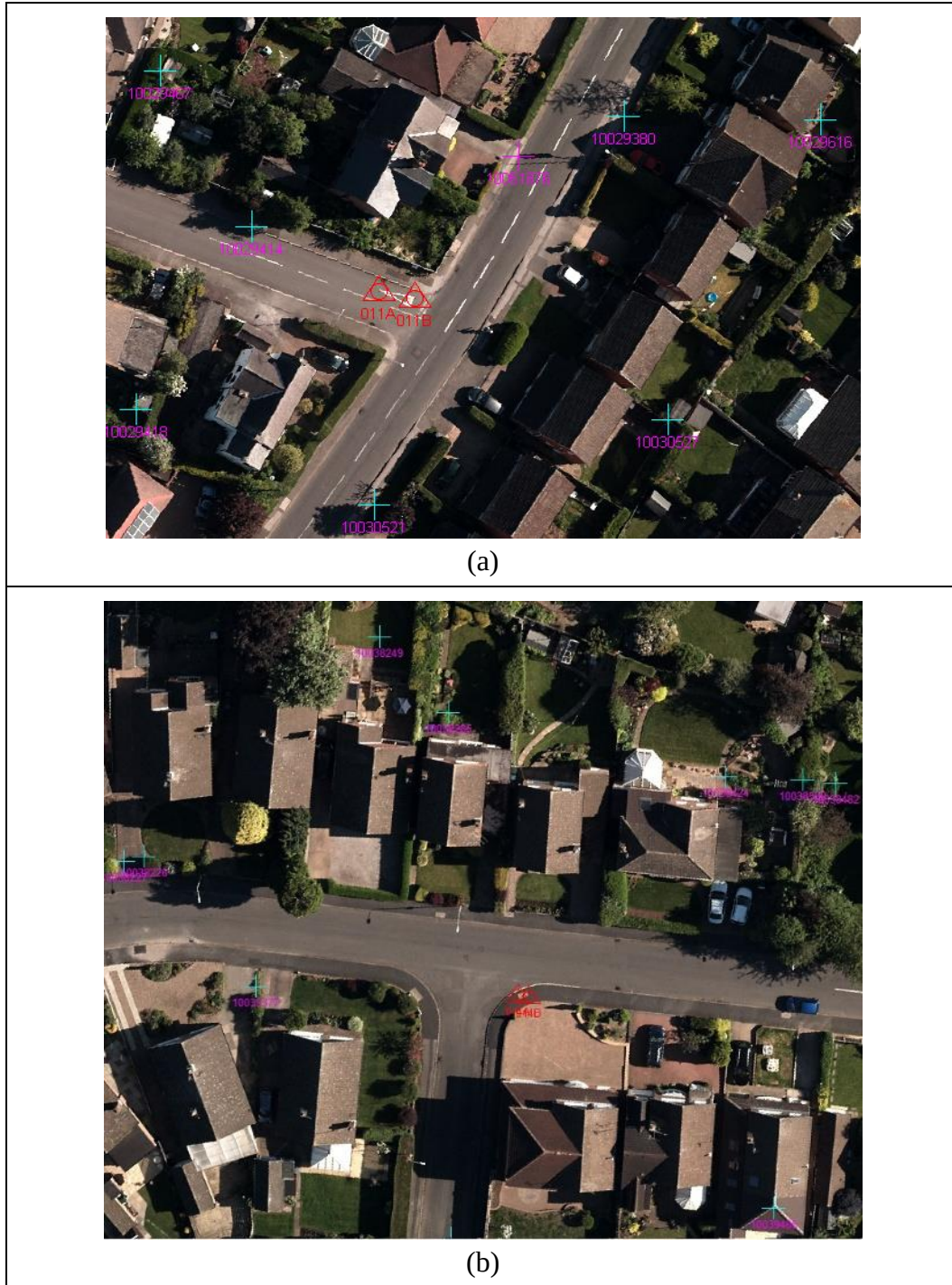
Figure 4.42: Close-up view of tie- (turquoise) and control points (red) in KN imagery
