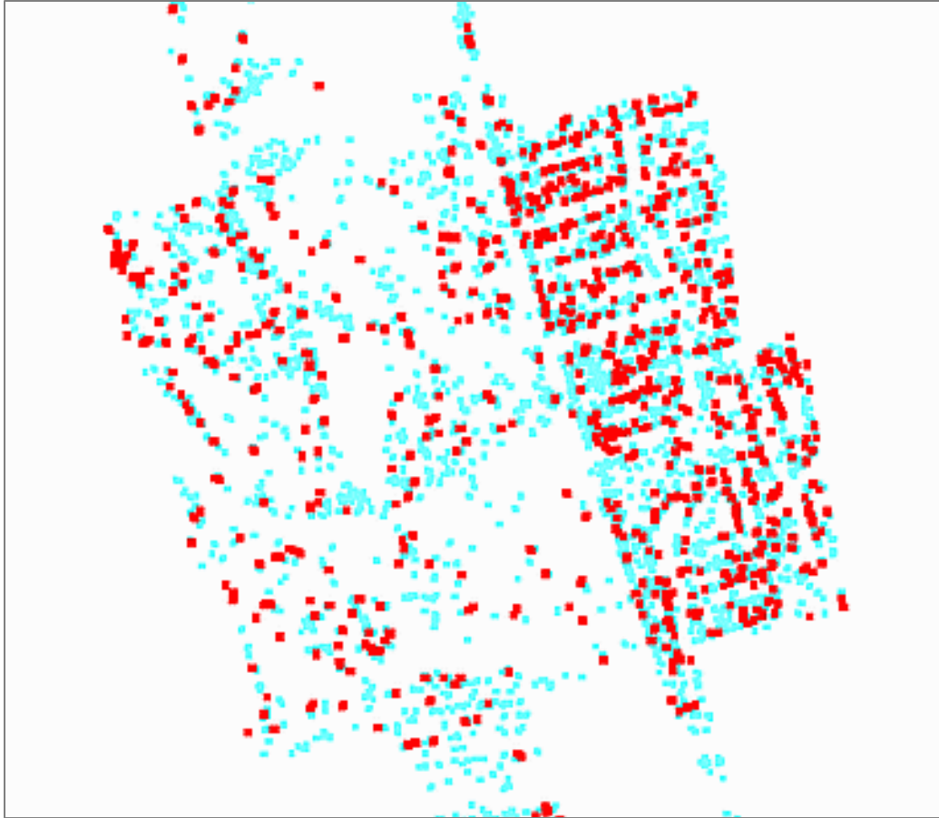
Figure 4.23: Automatically extracted tie planes in LMS software (Friess, 2006). Planes in red were included in the LSA
