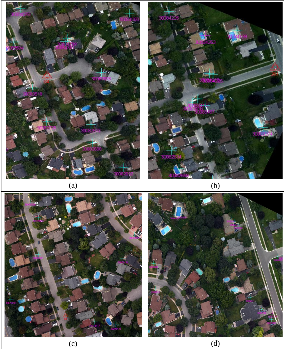
Figure 4.26: Examples of image-based tie points located at elevated corner locations and flat on the ground
