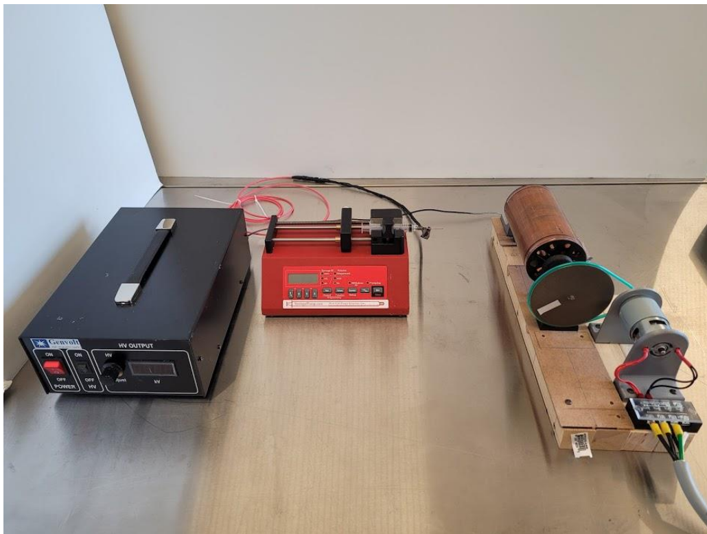
Figure 3-1 Overview of the components in the electrospinning setup
