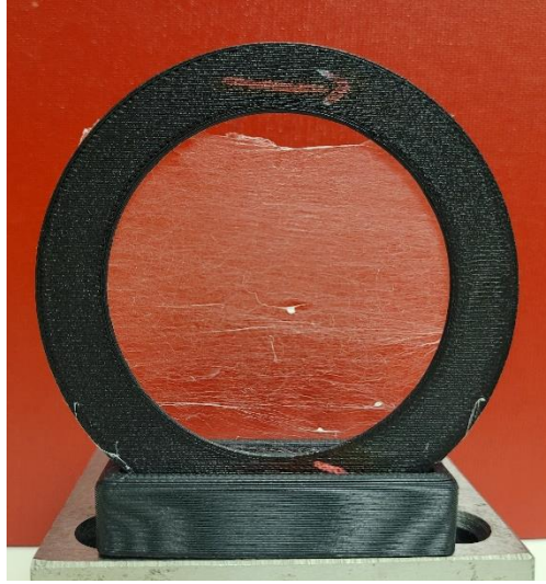
Figure 5-8 Torn nanofiber material mounted on plastic frame
