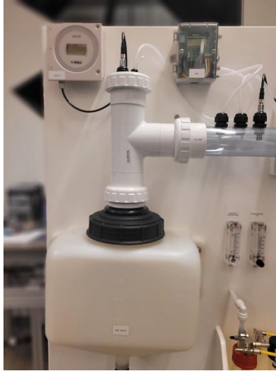
Figure 5-2 Buffer zone including the filter test stage with sensors before and after
