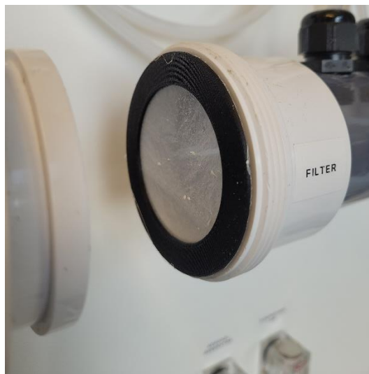
Figure 5-9 Mounted nanofiber frame in test apparatus
