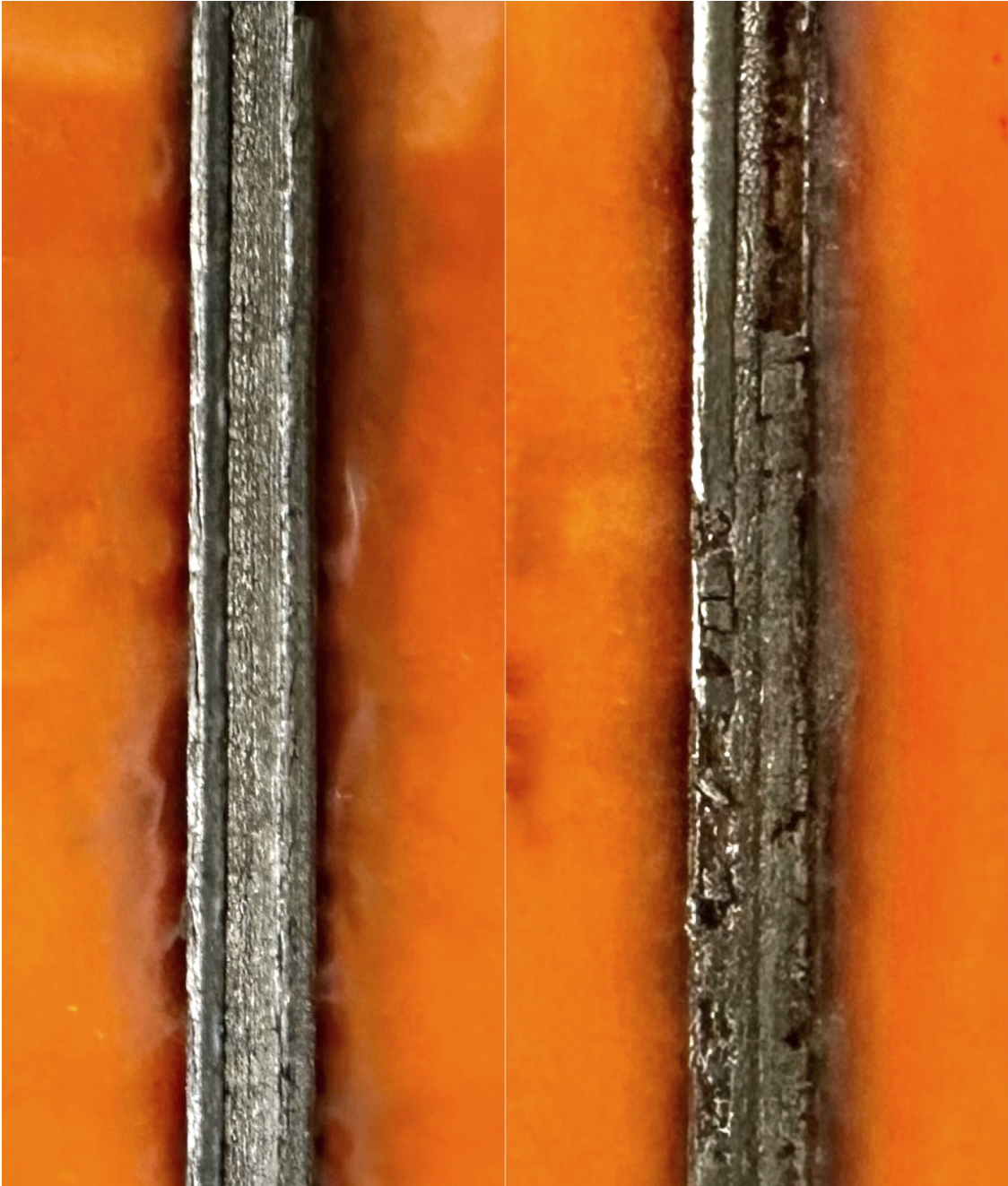
Figure 3.1: Effect of finger rubbing on the structure of a laser-induced graphene (LIG) sample. The left image shows the sample before rubbing, and the right image shows the sample after rubbing.
