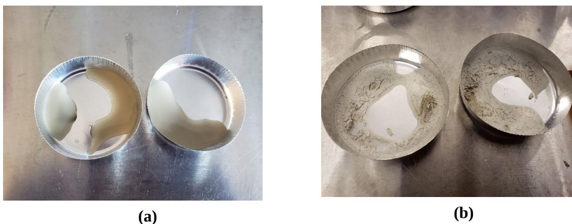
Figure 3.2 Estimating L:S of the bentonite stock solution (a) before oven-drying (b) after oven-drying.
