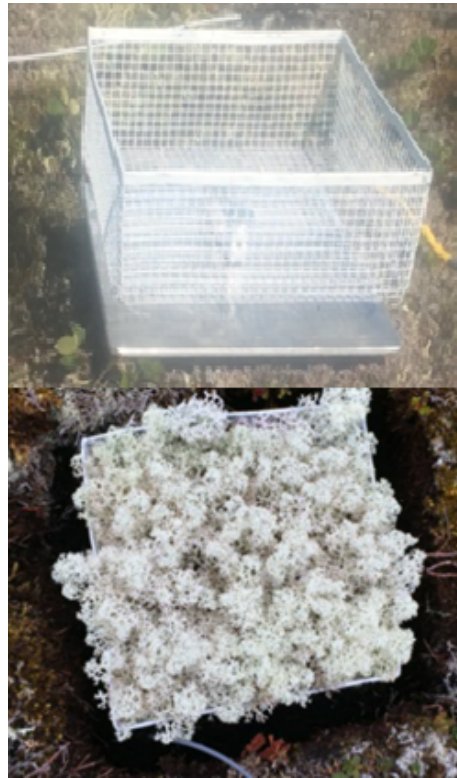
Figure 14: Top: An empty ¼" galvanized wire mesh basket, strain gauge and aluminum base plate prior to lichen placement. Bottom: Image with the lichen inside and installed in the peat.
