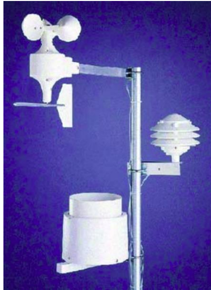
Figure 3.4 Typical Meteorological Sensors Installed on RWIS Stations (Source: www.gis.esri.com )
