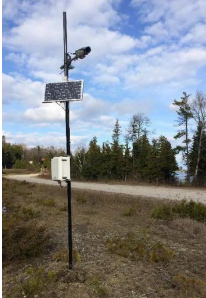
Figure 3.3 A Typical RWIS station (Source: Campbell Scientific Canada)
