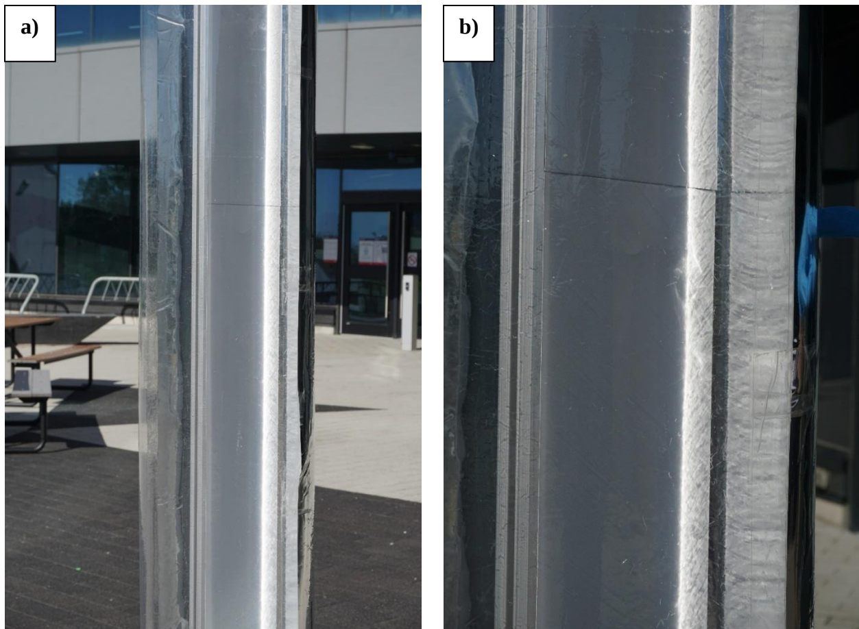
Figure 6.9. a) Lambertian target illuminated by concentrated sunlight and b) a close-up of the mid-region of the target. Photos were taken at 12:12:36 p.m. and 1:44:58 p.m., respectively.
