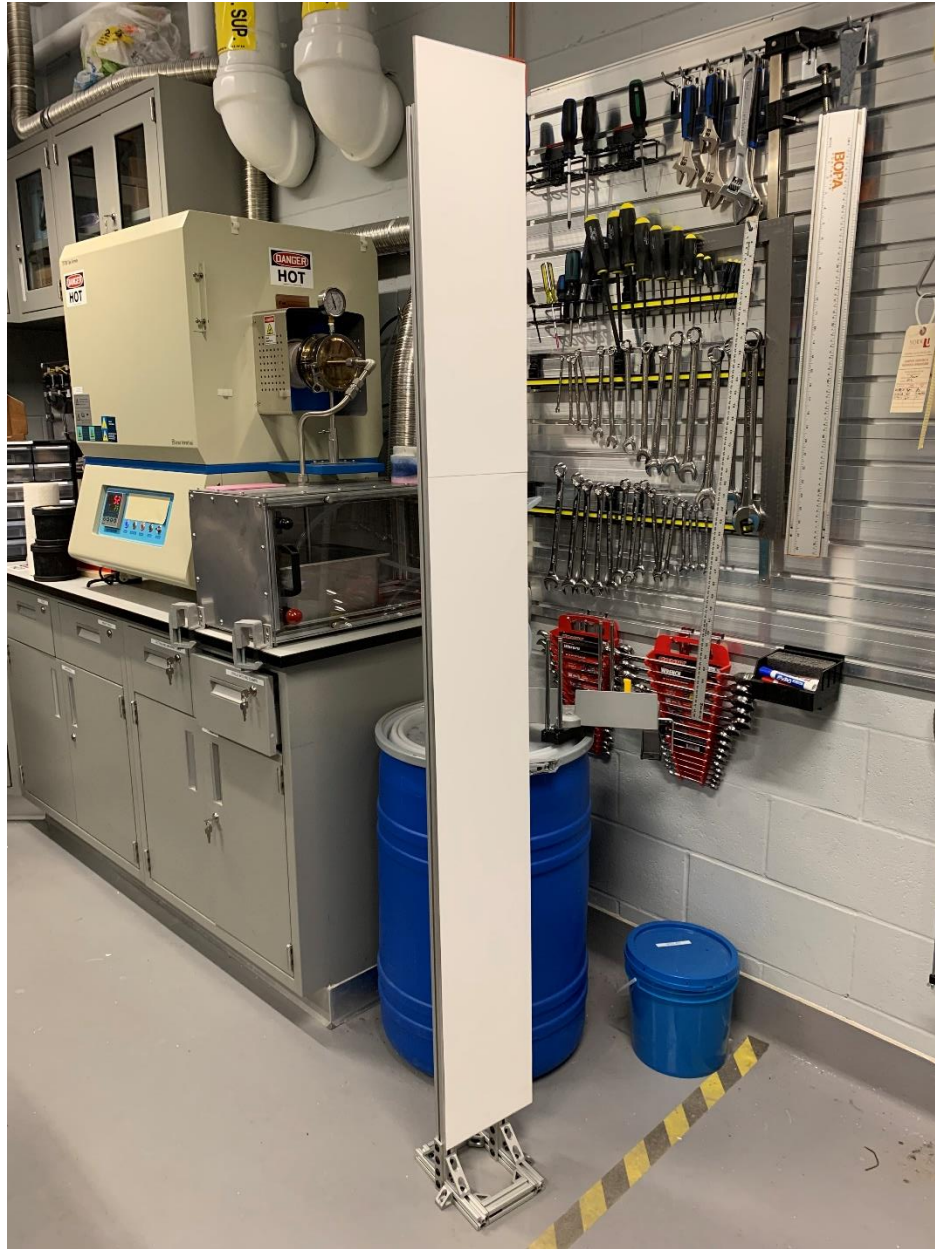
Figure 6.1. Lambertian target made of a 98% diffuse reflector film from WhiteOptics supported by aluminum framing. Due to the framing, the Lambertian target can only map 1 side of the mirror.
