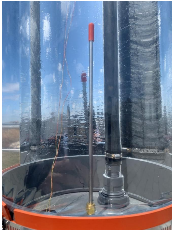
Figure 3.22. Aluminum tube (shadow stick) projecting a shadow onto the receiver indicating the collector is tracked.
