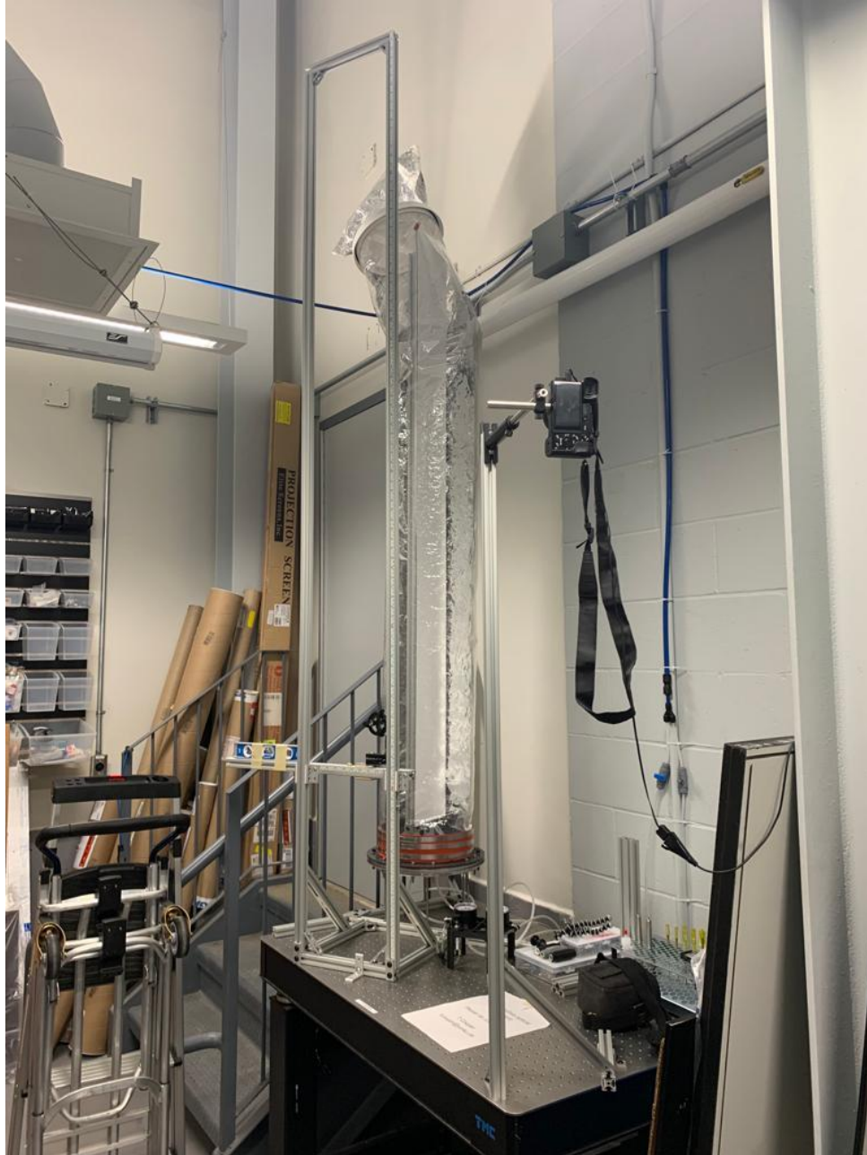
Figure 6.2. Experimental set-up for laser tests. The laser is mounted atop a track which slides both vertically and horizontally to fully define the system. A level is mounted to the cross member where the laser is fixed to ensure that it stays level with respect to the frame.
