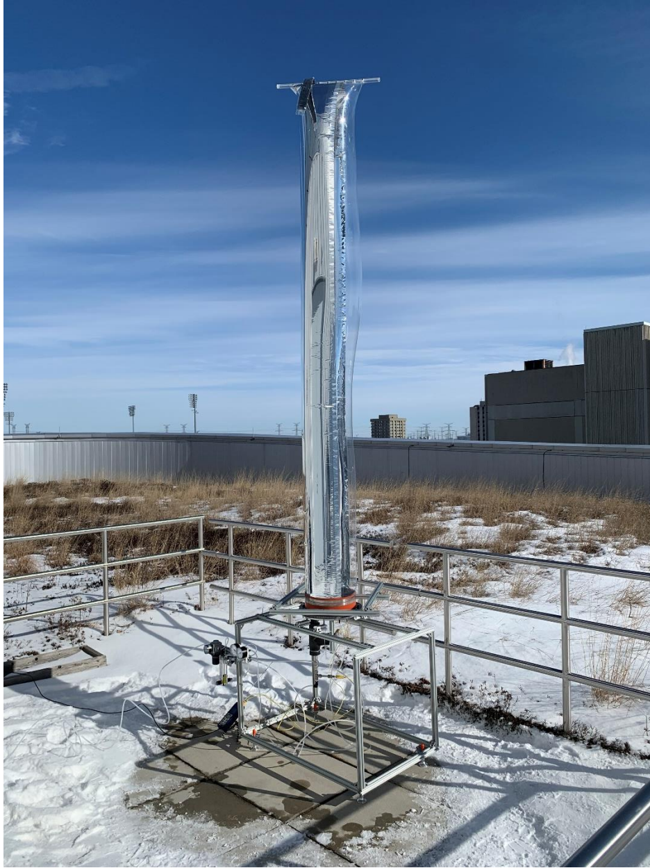
Figure 3.4. A vertical concentrator with a bag made from metallized polyester and ETFE experiencing plastic deformation due to the mismatch in the yield strength.
