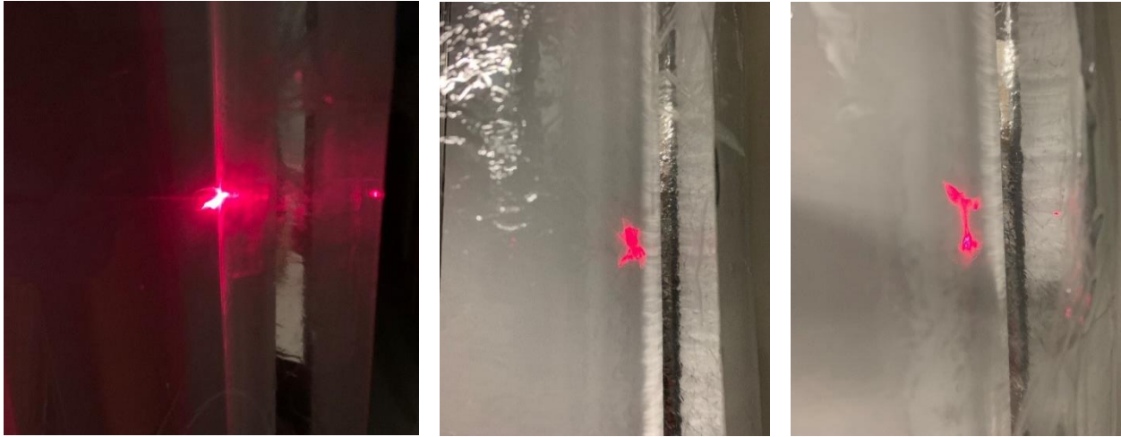
Figure 6.4. The effect of targeting regions of severe wrinkling.
