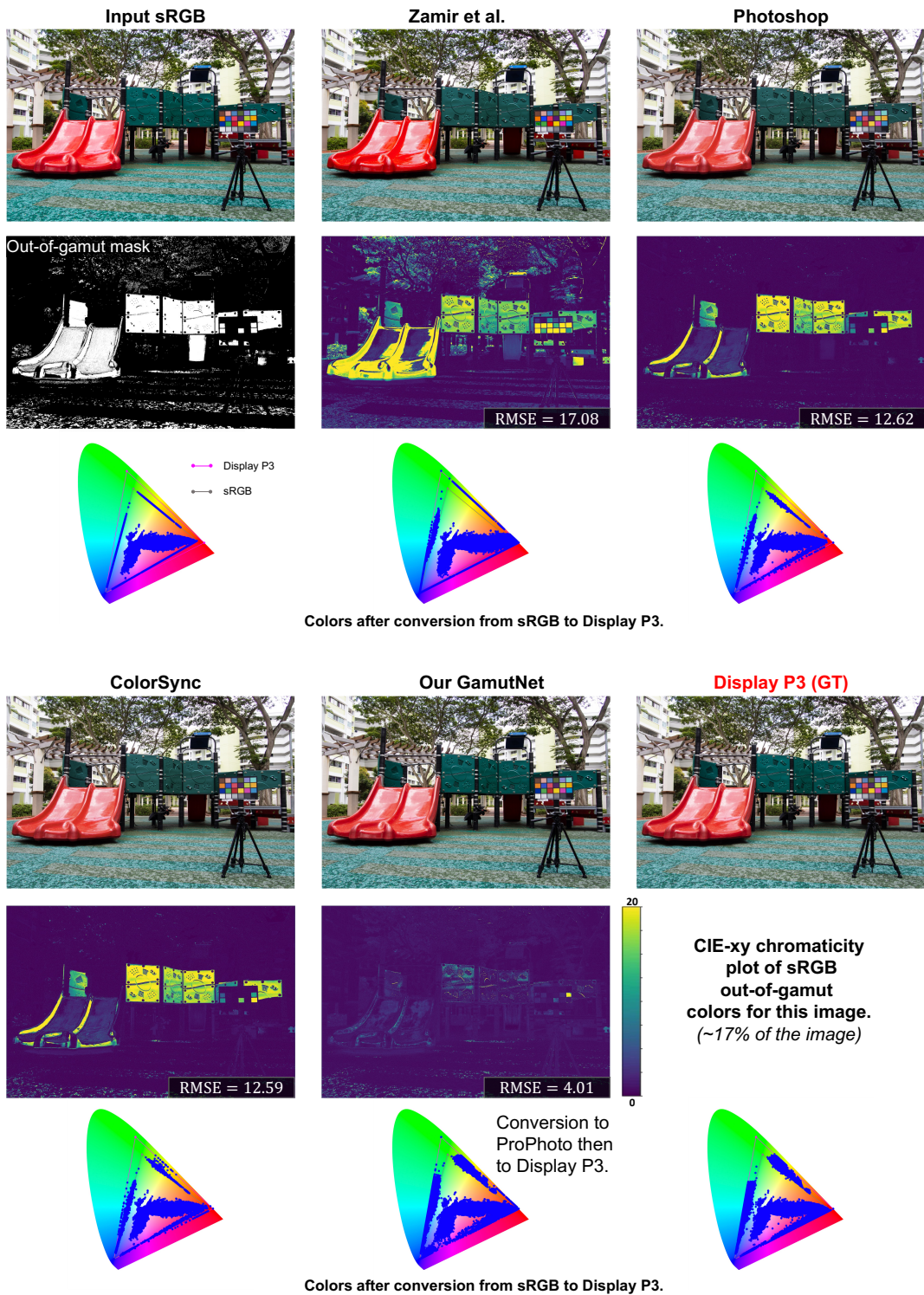
Figure 4.10: Comparisons among the Display P3 results of Zamir et al. [115] (gamut expansion), Photoshop [40], ColorSync [41], and our GamutNet. Heat maps of per-pixel RMSE are shown as well as plots of out-of-gamut colors on a CIE xy-chromaticity diagram showing the gamut for sRGB, and Display P3. GamutNet provides the best color space conversion.
