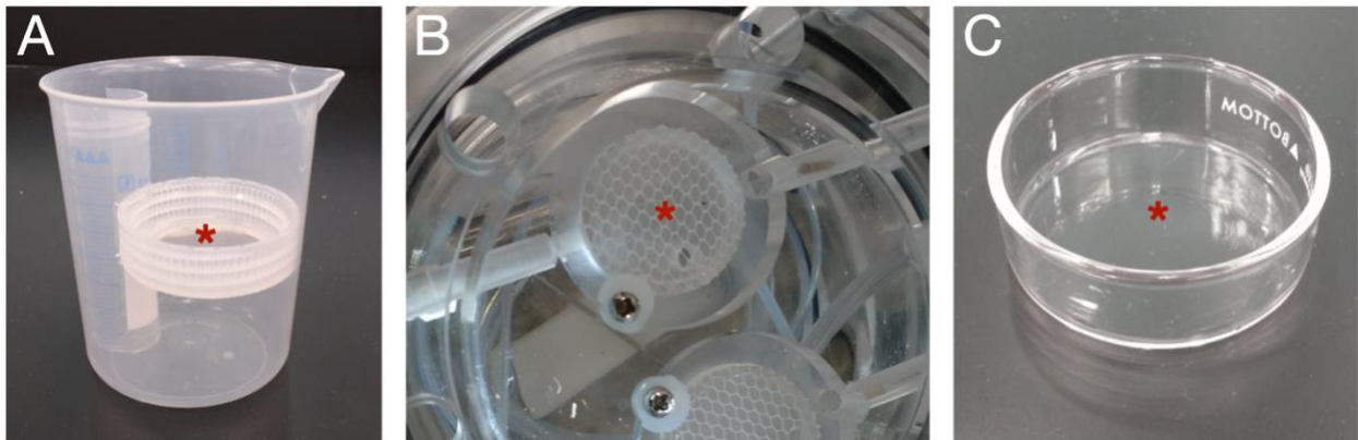
Figure 4.2.21: Options available for drug treatment incubation of hippocampal slices. The submersion chamber (A) holds slices 4-5 cm below the saline. The interface chamber (B) holds slices ~0.5 mm below the saline, and is used during the recording process as well. The glass Petri dish (C) holds the slices ~1 cm below the saline. Red asterisks denote the location of the slices during the incubation period.
