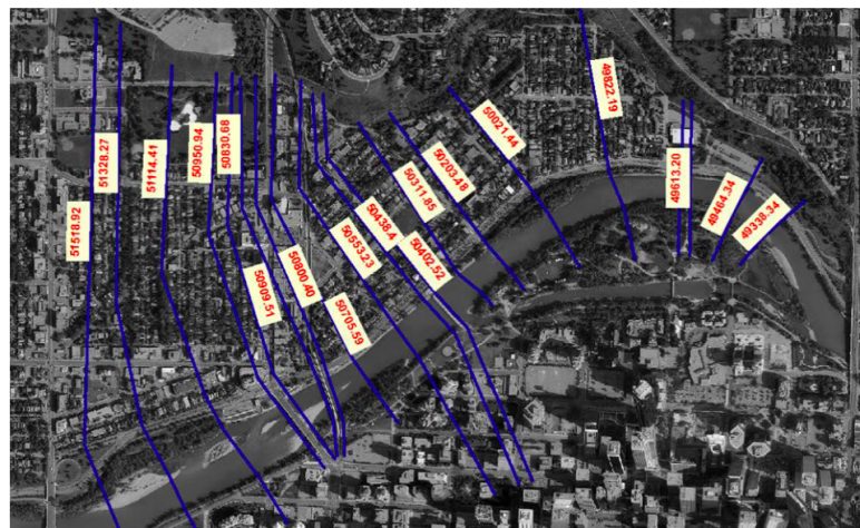
Figure 29: Levee cross-sections in the City of Calgary extracted from an HEC RAS model used by Cocaign et al., 2020
