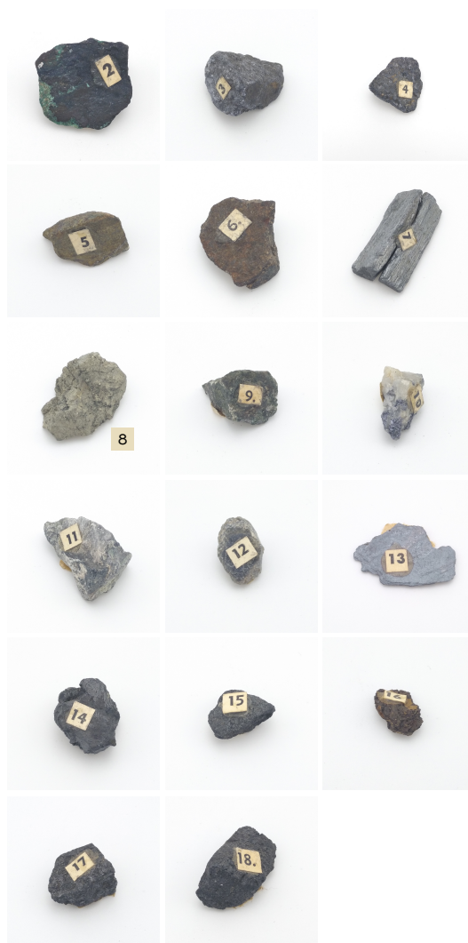
Figure 82: In numerical order from 2-18, the samples are chalcocite, galena, sphalerite, chalcopyrite, pyrrhotite, stibnite, pyrite, arsenopyrite, molybdenite (on gypsum), smaltite, corundum, hematite, ilmenite, pyrolusite, limonite, magnetite, and chromite.
