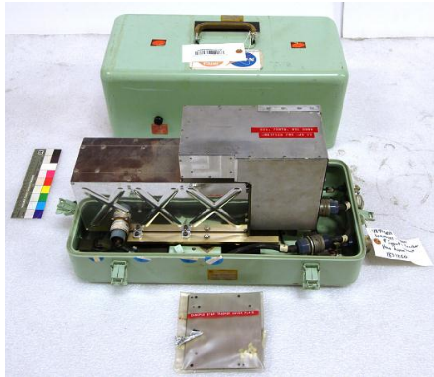
Figure 6 - Voyager Star Tracker and hood assembly. Image Credit: [11]
