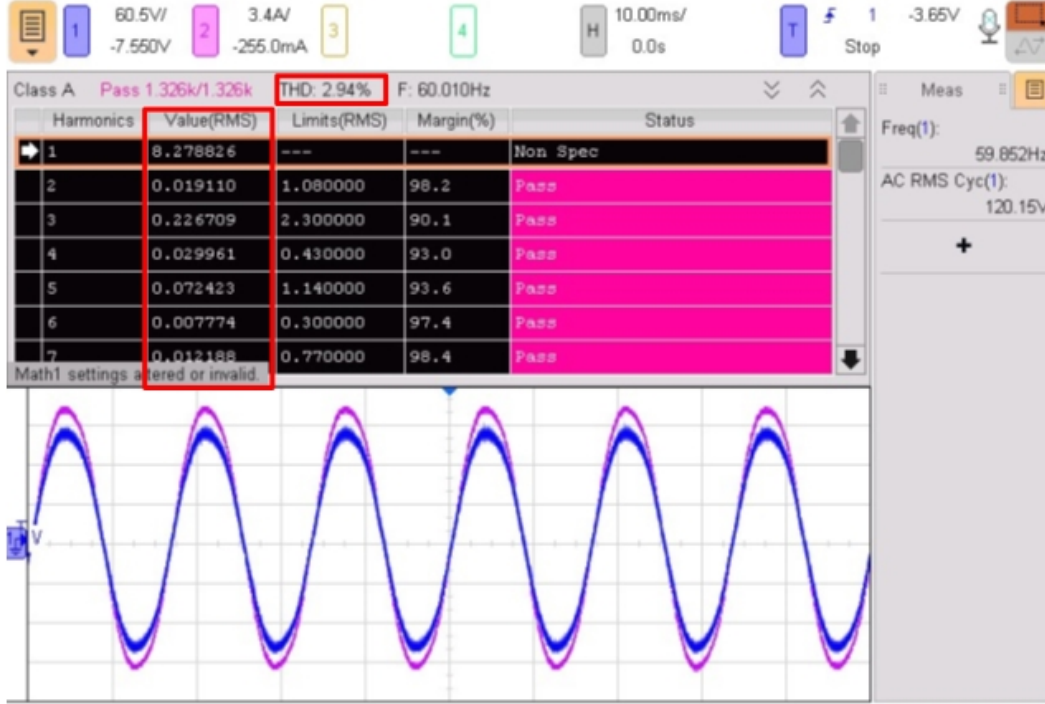
Figure 4.10: Experimental THD and output voltage waveform for L_{in} = 1 mH, showing 2.94% THD.
