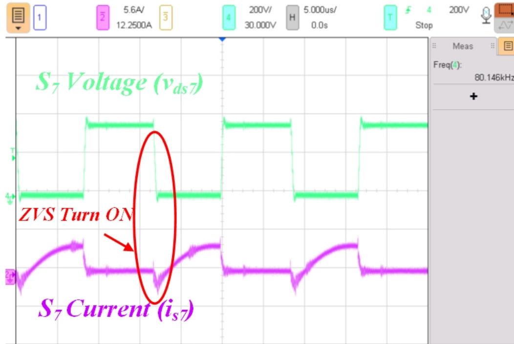
Figure 3.31: Voltage over and current flowing through S_7 at switching frequency in DC to AC mode.
