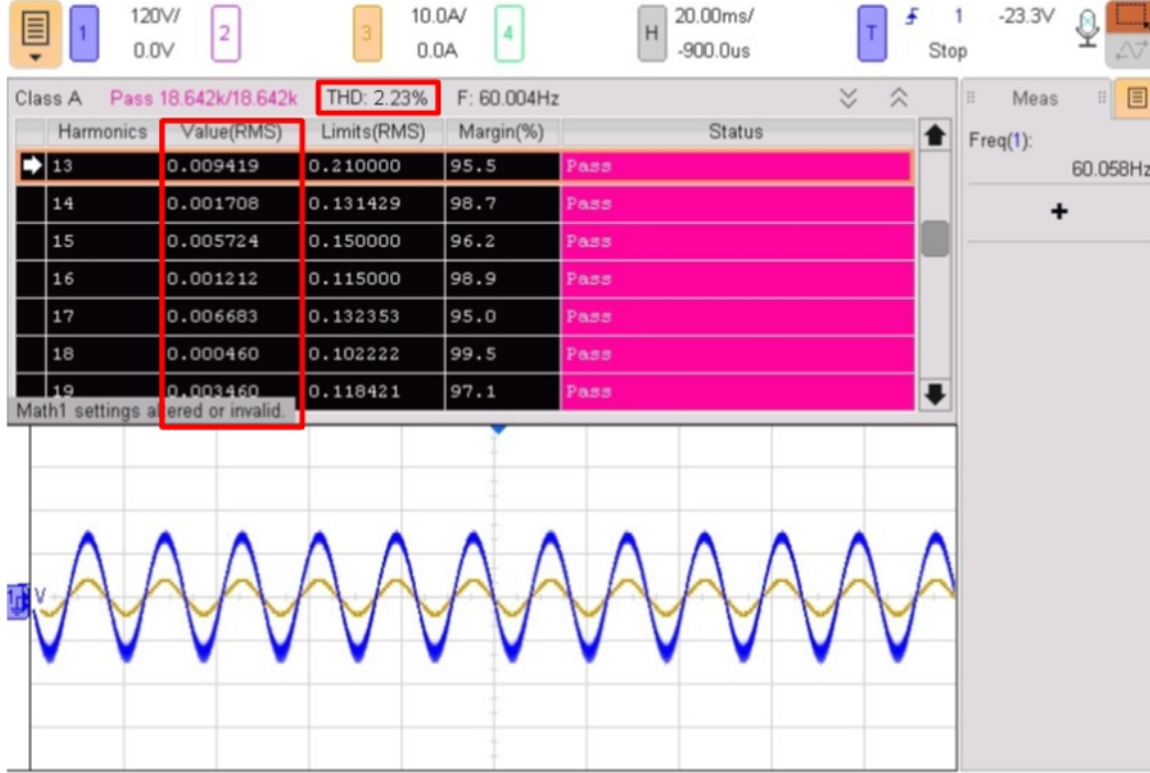
Figure 2.32: Harmonic distortion captured from the hardware experimental prototype showing thirteenth to nineteenth harmonics.
