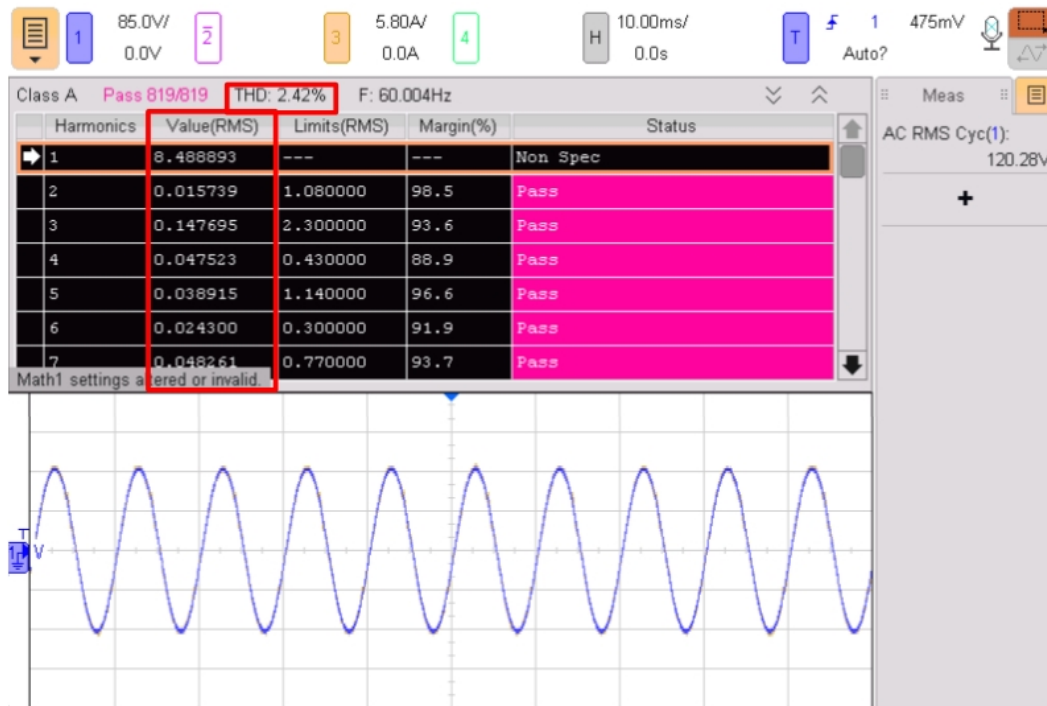
Figure 3.37: Harmonic distortion captured from the hardware experimental prototype
