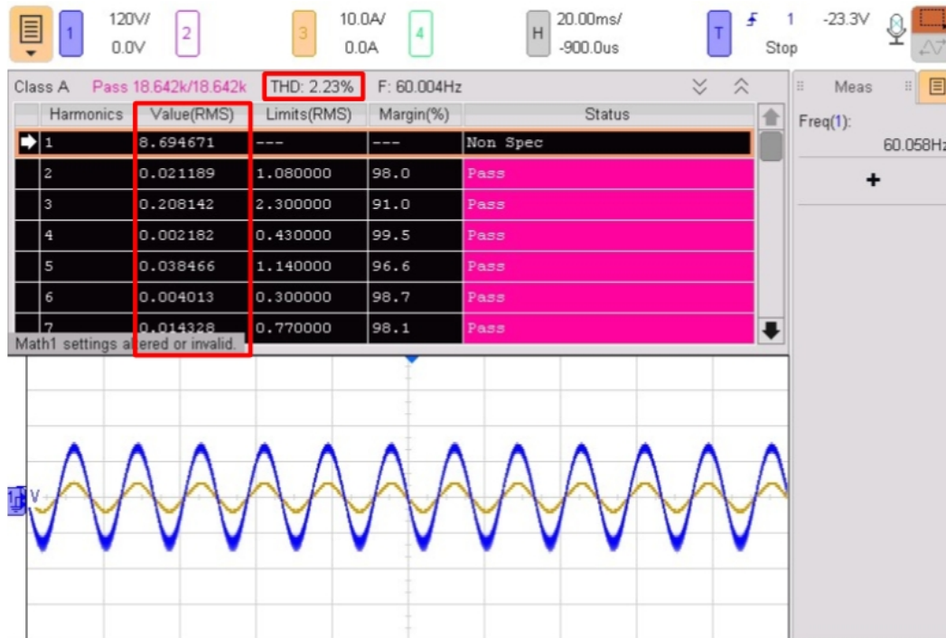
Figure 2.30: Harmonic distortion captured from the hardware experimental prototype showing first to seventh harmonics.
