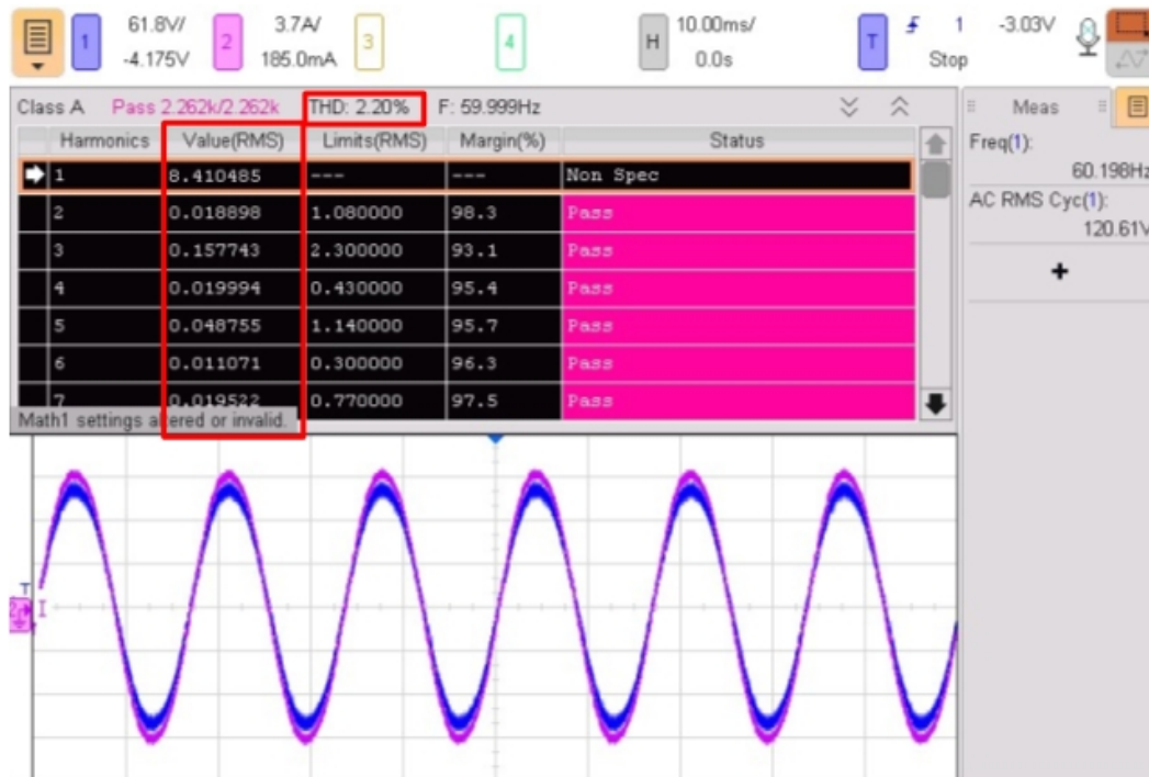
Figure 4.9: Experimental THD and output voltage waveform for nominal case L_{in} = 550 \mu\text{H} , showing 2.20% THD.
