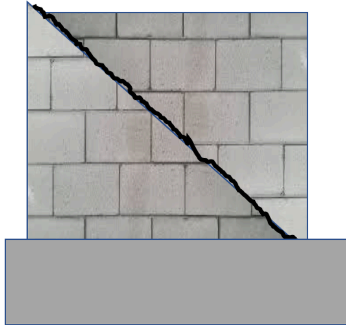
Figure 2.6) Illustration of the diagonal failure of a reinforced masonry wall that has failed due diagonal tension from the yielding of horizontal reinforcement
