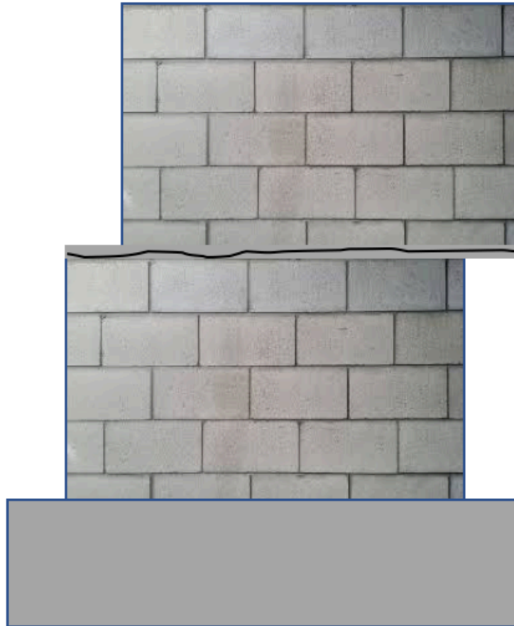
Figure 2.4) Illustration of a typical sliding plane of a reinforced masonry wall that has failed due to sliding along the mortar-brick interface
