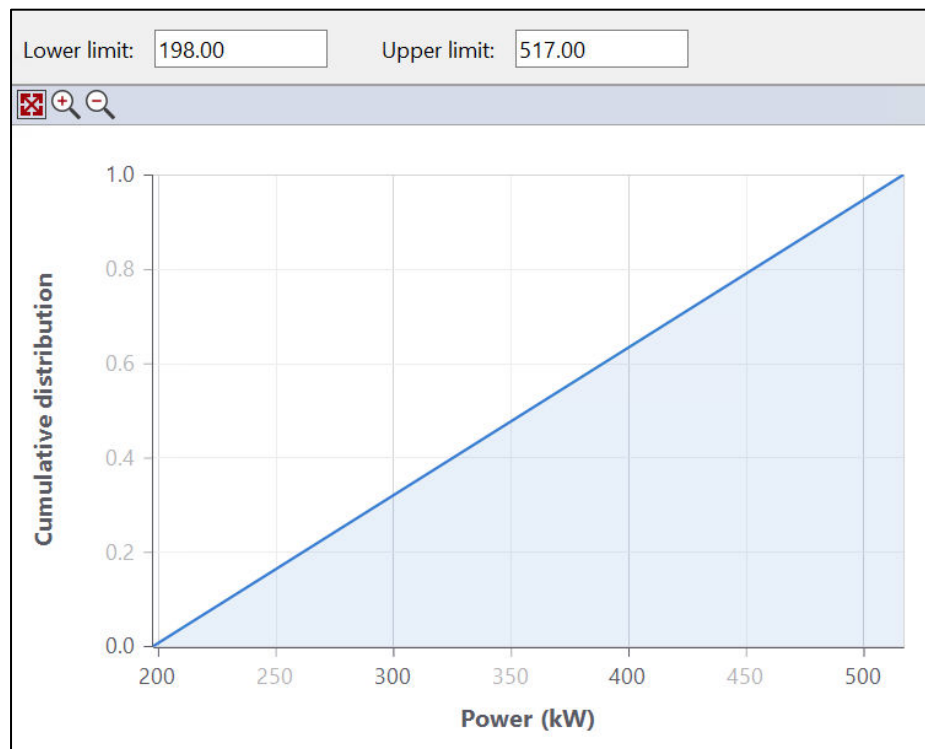
Figure 28: Heavy Goods Vehicle Power Distribution in Vissim
