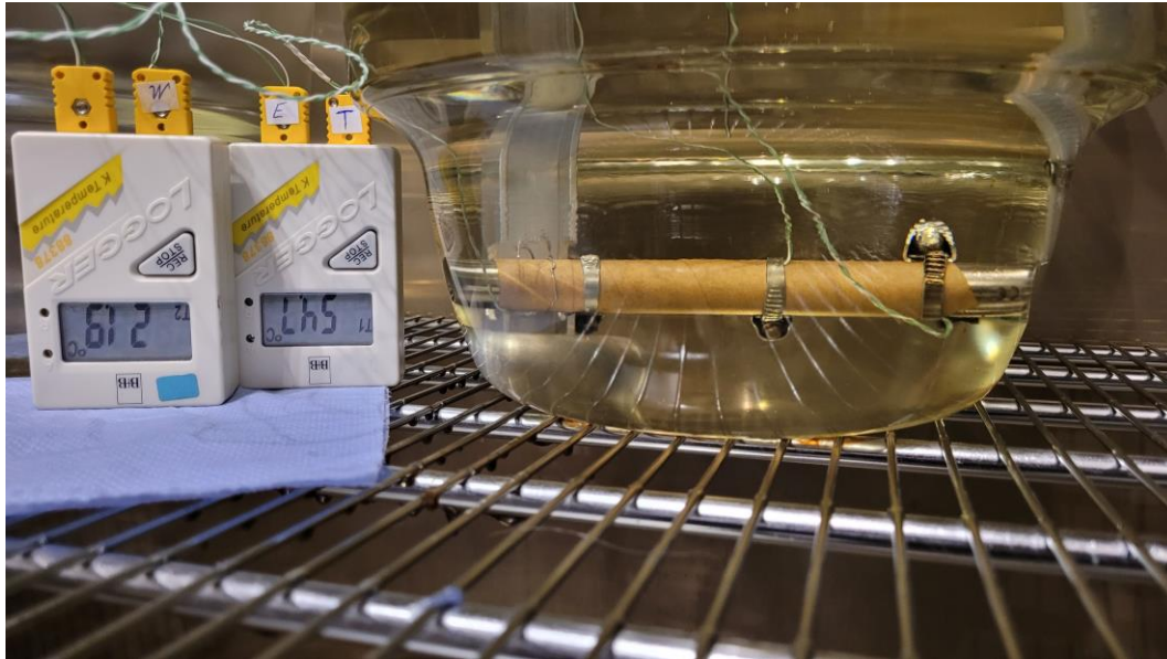
Figure 4-5: Glass vessel with the cartridge heater immersed in the oil.
