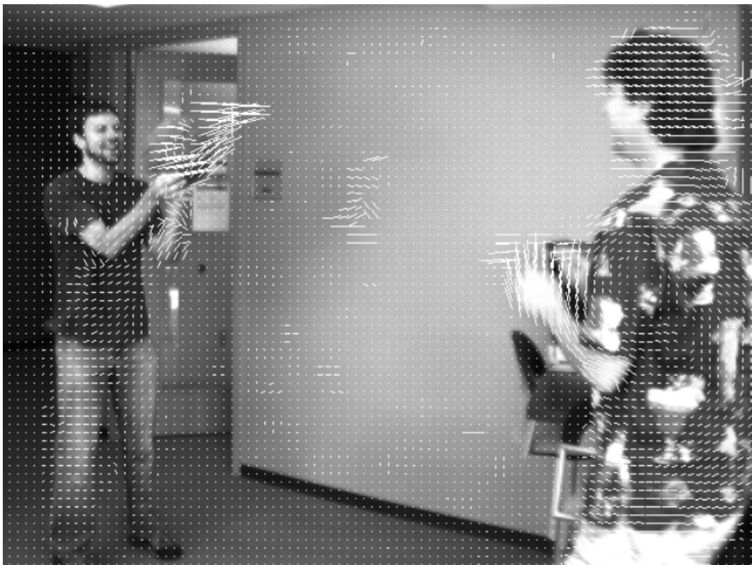
Figure 2.2: Graphic of optical flow vectors overlaid on a greyscale image.[2]
