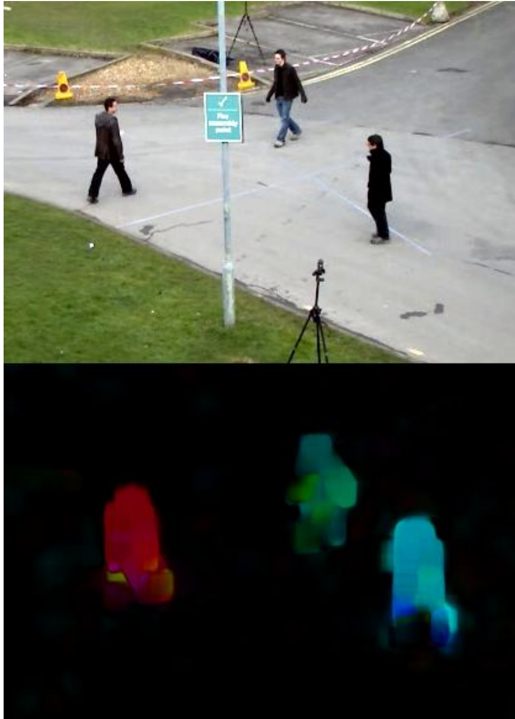
Figure 2.3: Figure 1. Visualization of dense optical flow using OpenCV.[3]
