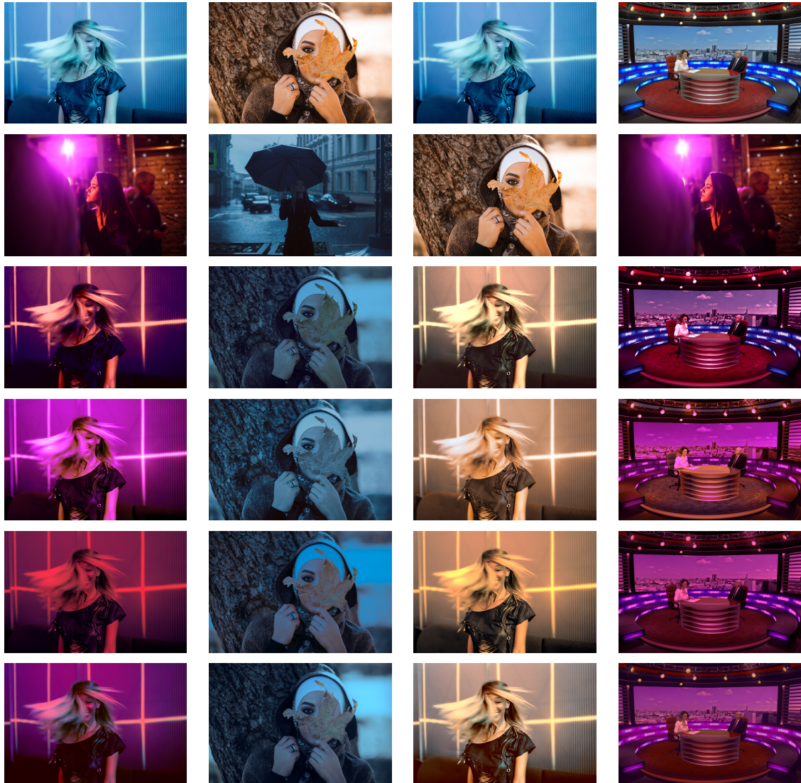
Figure 5.6: From top to bottom, sources, targets, proposed result, Grogan result [14], Photoshop result [15], and Zabaleta & Bertalmío result [16].
