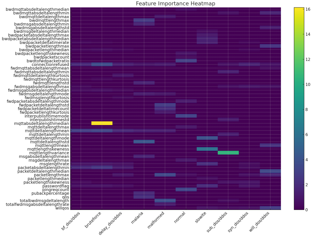
Figure 24: Heatmap of class-wise local feature importance based on TabNet’s attention mechanism. Brighter cells denote a higher influence of the corresponding feature for that class.
