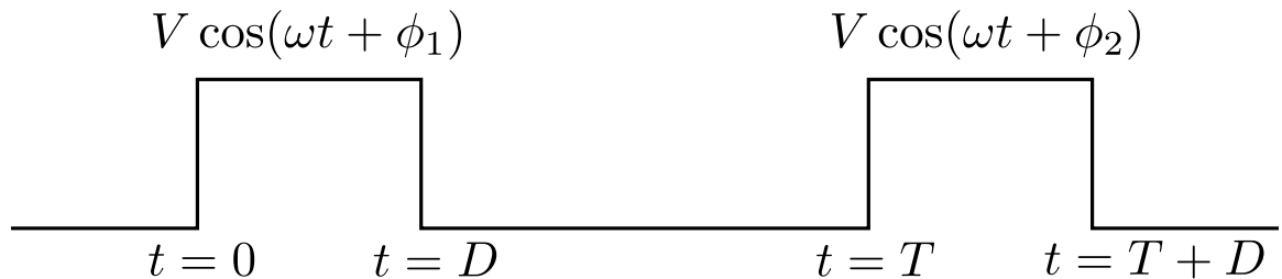
Figure 2.1: Timing diagram for microwave pulses in the Separated Oscillatory Fields (SOF) and Frequency-Offset Separated Oscillatory Fields (FOSOF) techniques. The pulses are of duration D and their starting edges are separated by a time T .
