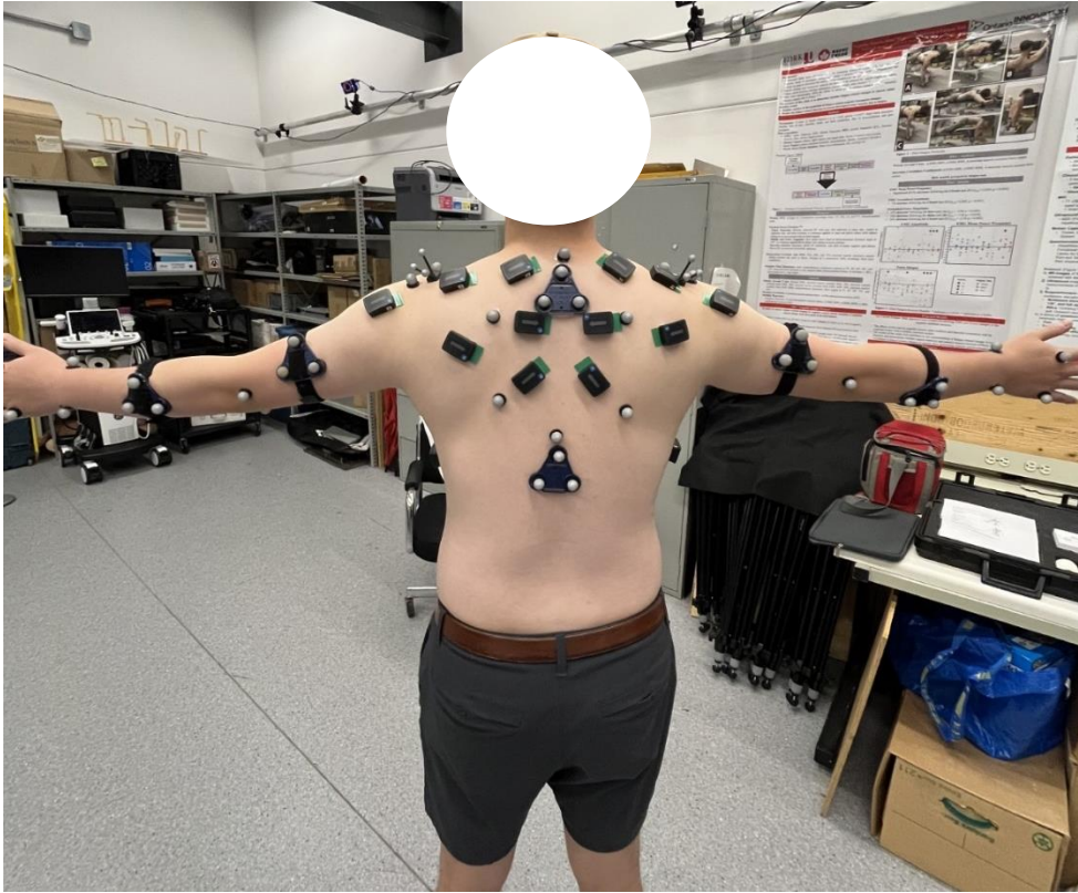
Figure 4. Protocol set up demonstration, with participants having placed Delsys EMG wireless electrodes. Scapulothoracic kinematic reflective markers placed in single marker form, triangle cluster form, and scapular tracking cluster form.
