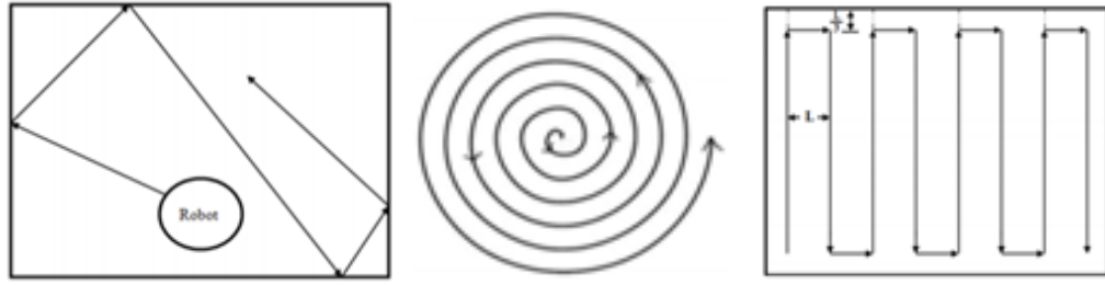
Figure 2.2 Motion path of RW, spiral, and S-shape algorithms [18]
