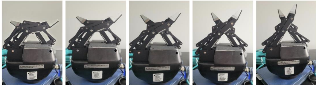
Figure 3.8 Robotiq 3-Finger Gripper Movement
