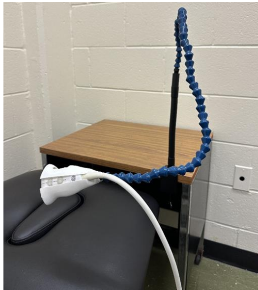
Figure 5. Ultrasound transducer housed by transducer holder / jig.
