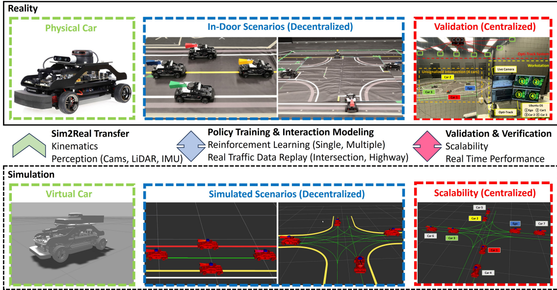
Figure 2.2: Leveraging computer simulations to improve real-world AD performance using three types of techniques: sim-to-real, self-play training, and algorithm validation.
