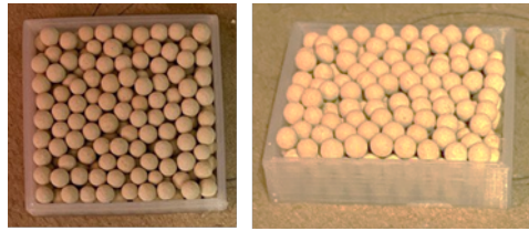
Figure 5.1 Zeolite 13X samples placed inside 3D printed Poly-lactic Acid (PLA) frames.
