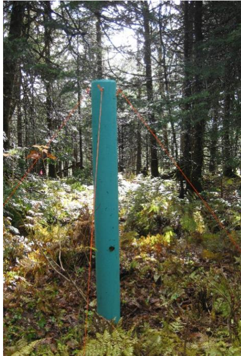
Figure B-5: A photographic example of a custom-built Polyvinyl Chloride (PVC) static sampler, which was deployed at the NL-BELT field sites for the entire sampling campaign. Nylon ropes secured to rebar anchors are used to keep the sampler upright while also possible to break if interacting with large wildlife (e.g. moose) in the region without causing injury.
