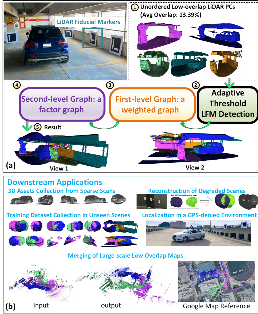
Figure 4.1: An overview of the proposed framework for mapping and localization using LFM.
