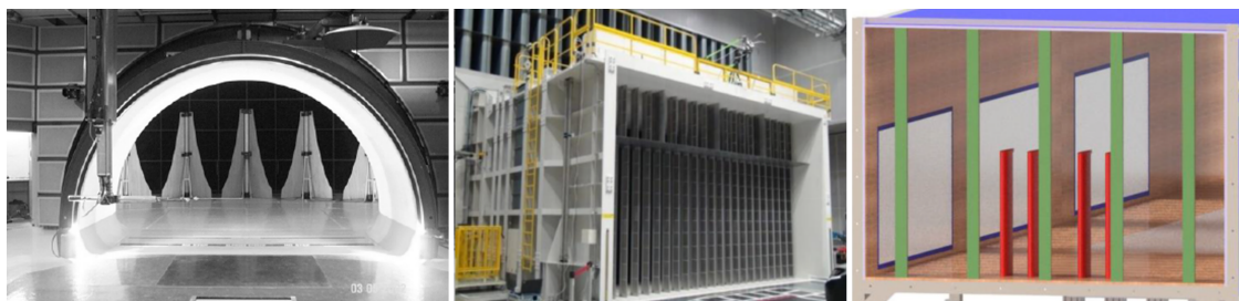
Figure 2.3: Pininfarina active drag-based TGS (left) [11], Toyota active lift-based TGS with shutter system (middle) [10], FKFS Active Flaps lift-based TGS with passive bars (right) [28]. Reprinted with permissions.
