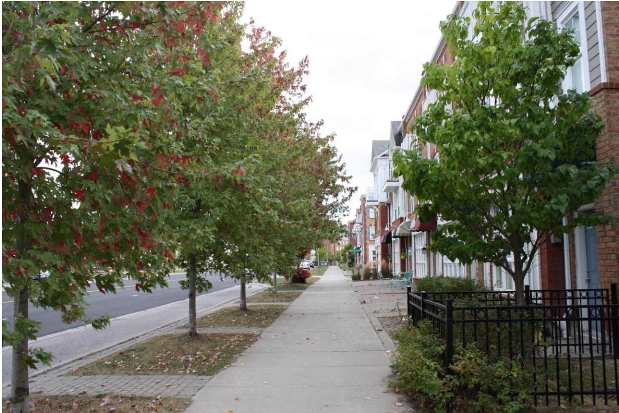
Figure 23: Pedestrian sidewalk along Bur Oak Avenue - From left to right: Bur Oak Avenue, on street parallel parking, boulevard with tree plantings, wide sidewalks, porches, mixed-use buildings. Source: Victoria Moore (September 28, 2017)
