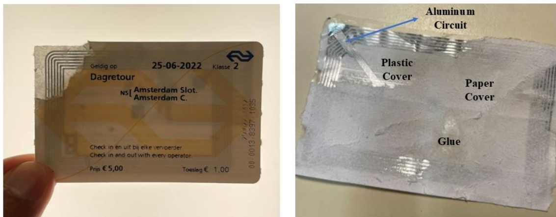
Figure 6.1 Transportation tickets with an integrated RFID antenna tag made of various materials.
