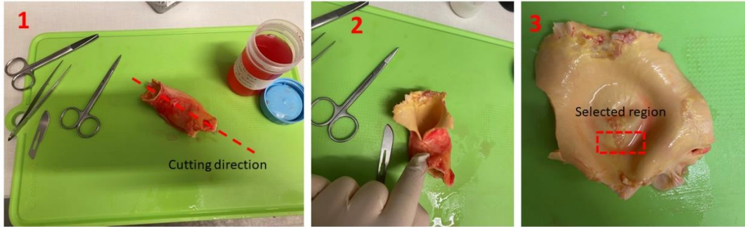
Figure 28. The procedure of preparing the aorta sample. Cutting the aorta sample in 3 steps with a dissection scissor and a surgery knife.
