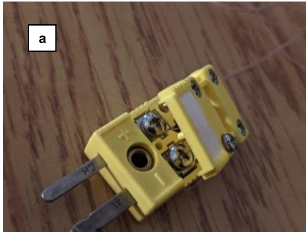
Figure 3-14: (a) K-type thermocouple from Omega Engineering; and (b) dismantled K-type Thermocouple using a precision screwdriver, showing interior components, including: two screws, bearing, thermocouple wire made of chromel/alumel (nickel alloys of the respective metals) with grommet.
