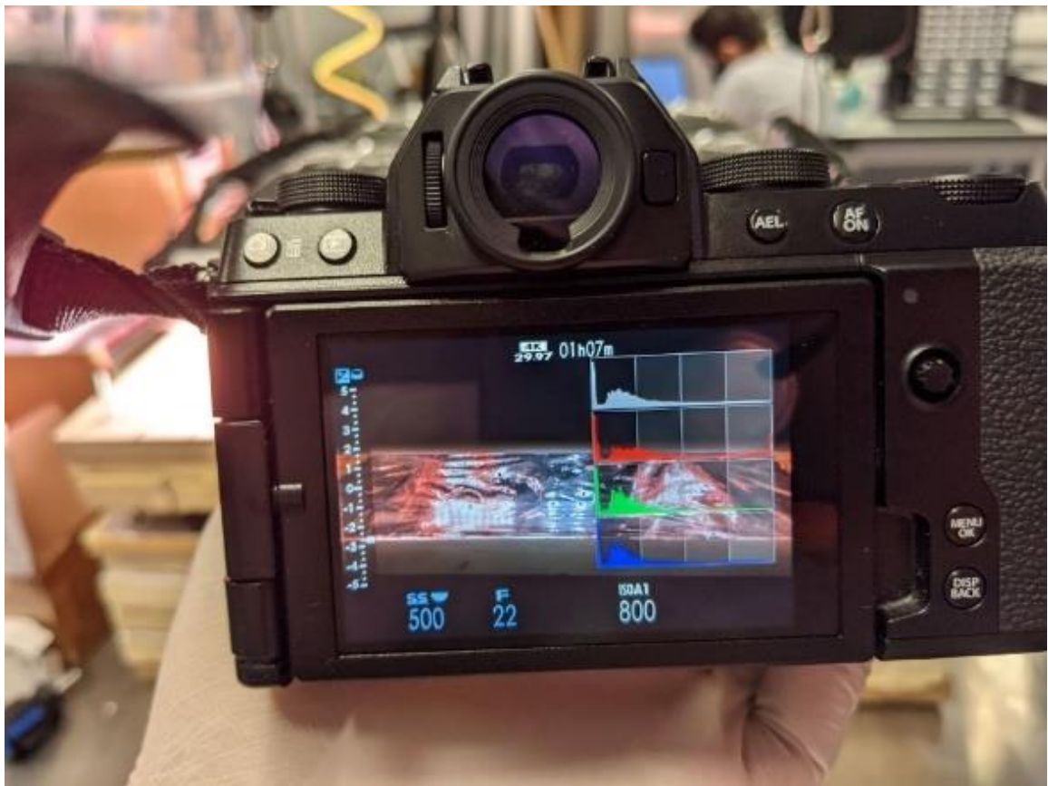
Figure 3-23: Camera histogram used to ensure properly exposed photographs during flux map images taken.
