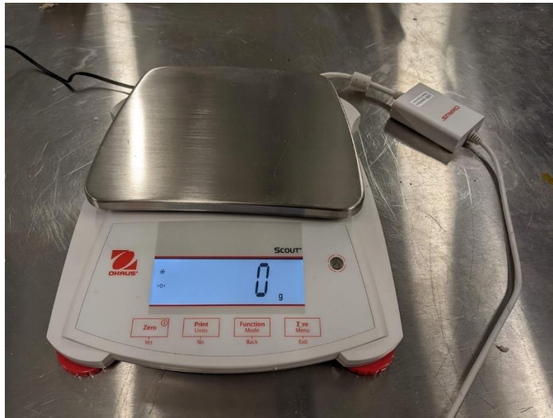
Figure 3-30: Picture of OHAUS Scout Mass Balance connected to a USB logger (logged to OHAUS software on computer).
