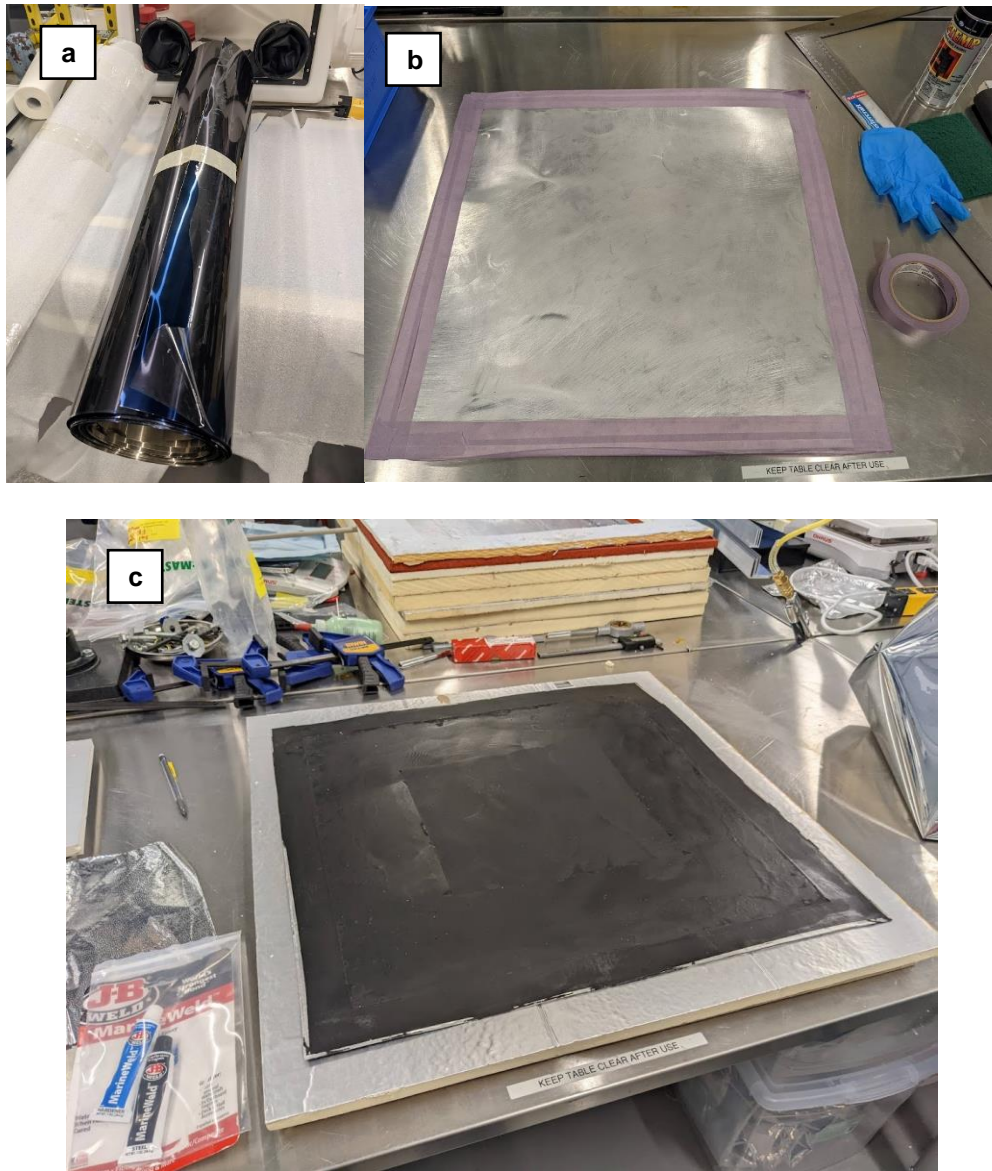
Figure 3-8: (a) Large roll of solar selective absorber to be cut and uncurled. (b) After cutting an 18 inch x 18 inch piece, selective surface is uncurled, sanded and masking taped at sides to avoid epoxy spillage on absorbing side. (c) Finally, it is spray painted.
