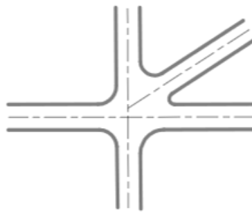
Figure 16 Multi-legged intersection (TAC, 2017)
