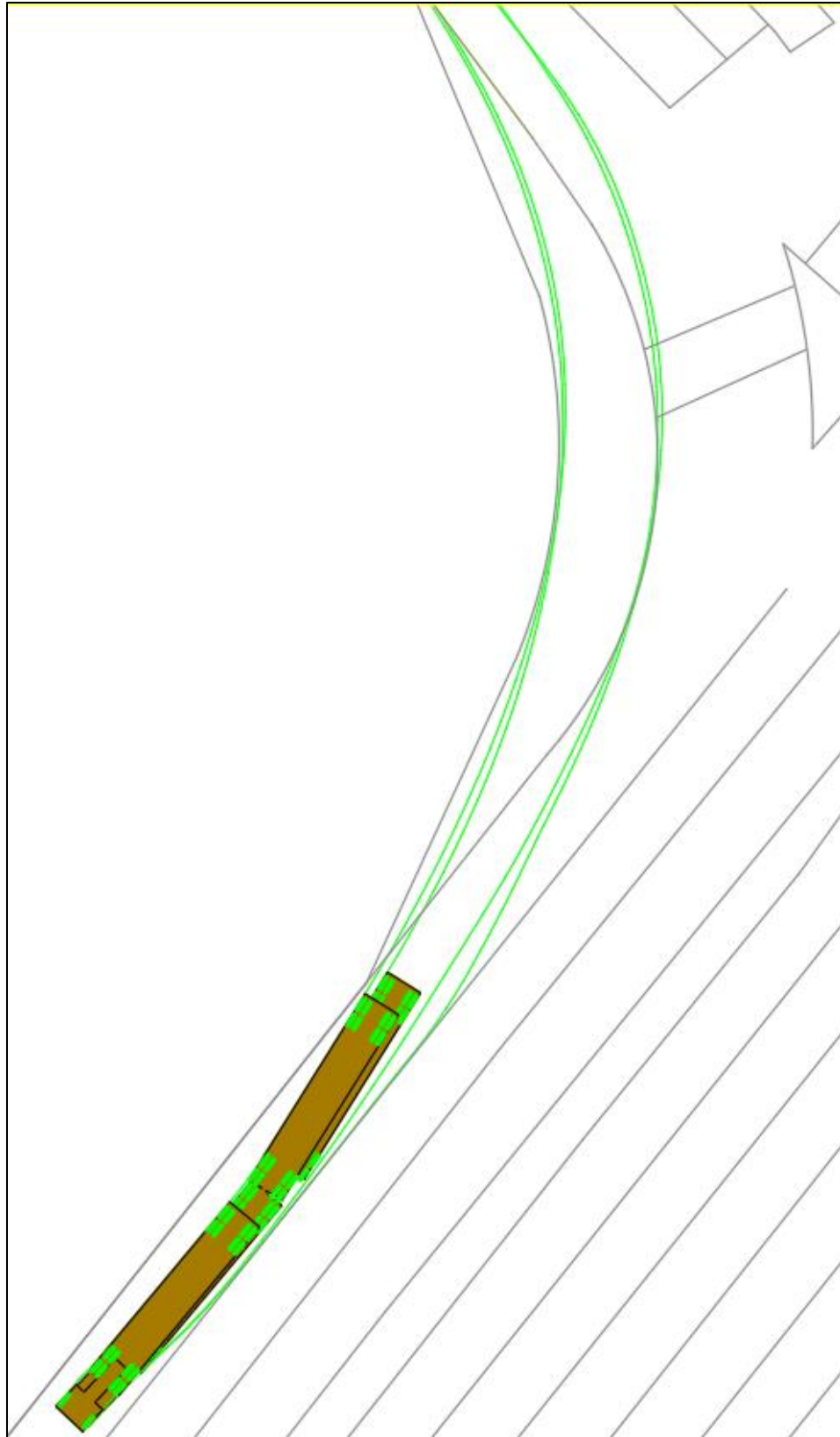
Figure 23 Overlaid swept paths (in green) for conventional and cabover tractors
