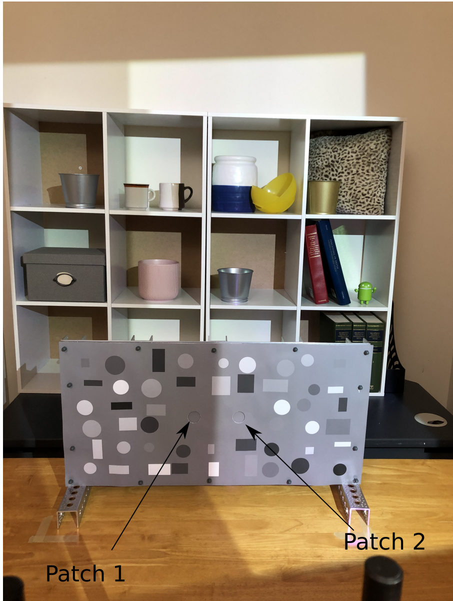
Figure 7. Apparatus for Experiment 1. The grey background is populated with multiple circles and rectangles with different reflectance values. The circles indicated by arrows represent the locations of the test and reference patches.
