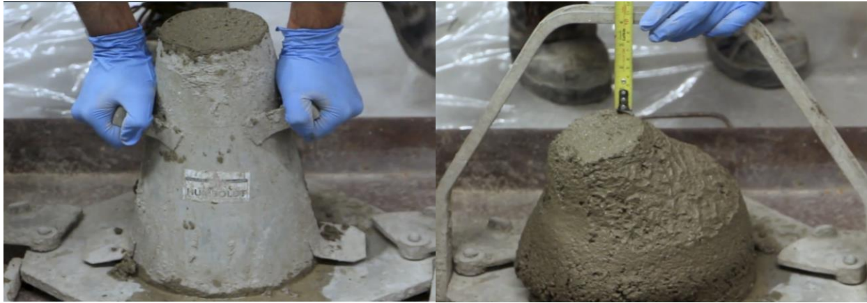
(a) (b) Figure 43-Visualization of concrete slump test
