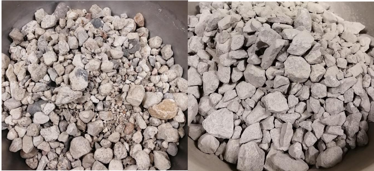
(a) (b) Figure 2-Coarse Aggregates, (a) Coarse RCA (CRCA), (b) Coarse NA (NCA)
