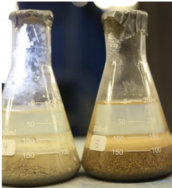
Figure 42-Total absorbed moisture with time after 2 weeks [Left]-FRCA [Right]-NFA
