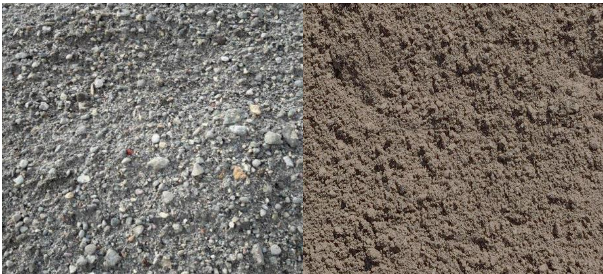
(a) (b) Figure 3-Fine Aggregates, (a) Fine RCA (FRCA), (b) Fine NA (NFA), natural sand
