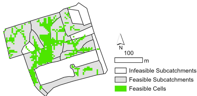
Figure 4.9 The location of feasible subcatchments (the area of feasible cells within the catchment is greater than 5 % of the area of catchment)
