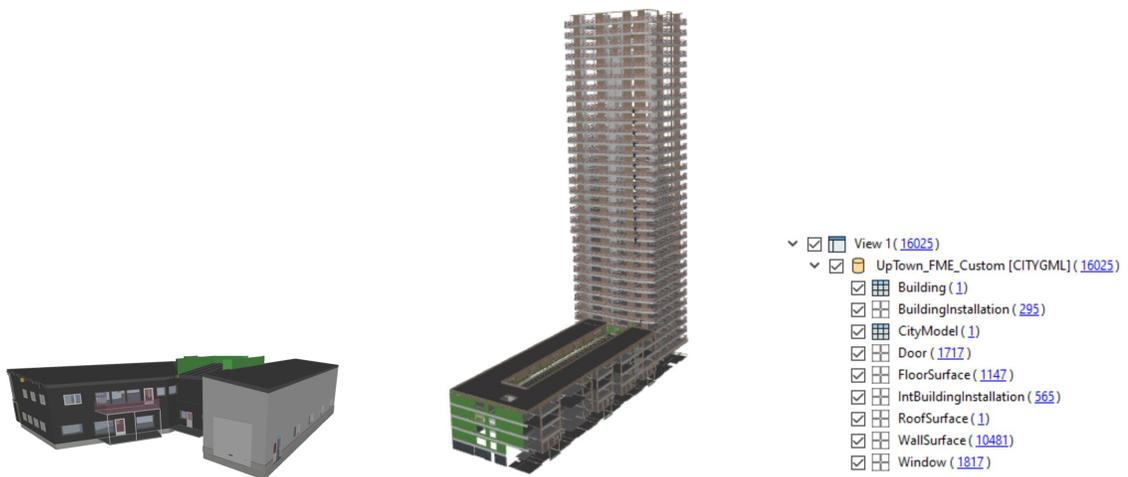
Figure 4.8: Conversion results of IFC data into LoD4 CityGML models using FME Workbench where limited features were transformed, and related semantics (attributes, entity types and hierarchy) were kept with respective CityGML feature types.
