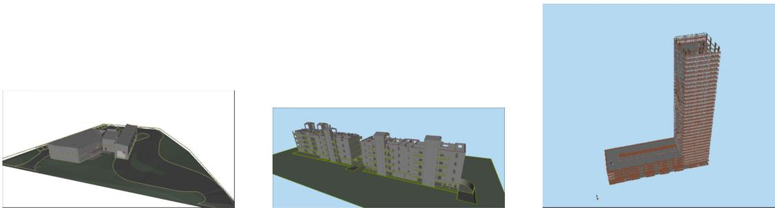
Figure 4.5: Quick translation results of IFC data into LoD4 CityGML models where not all geometries were transformed, and minimal semantics were kept with CityGML *GenericCityObject* feature type.
