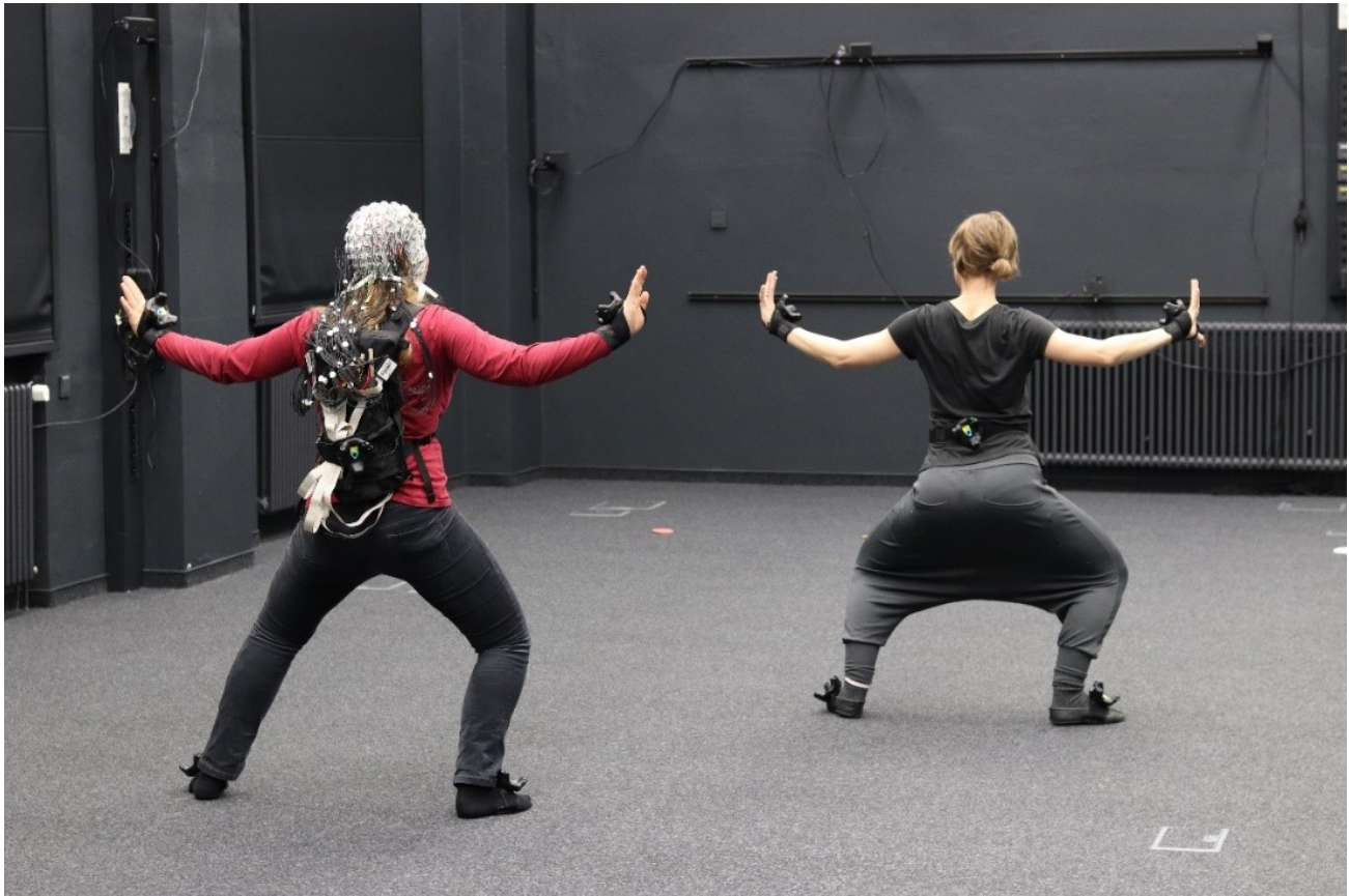
Figure 2: LEARN trial with the teacher; subject is wearing an ActiCap with 128 active electrodes (Brain Products); both subject and teacher are wearing 5 Vive Motion capture pucks (HTC Vive): 2 each on wrists and ankles, and 1 on the centre of the back. Pictures courtesy Benjamin Paulisch.
