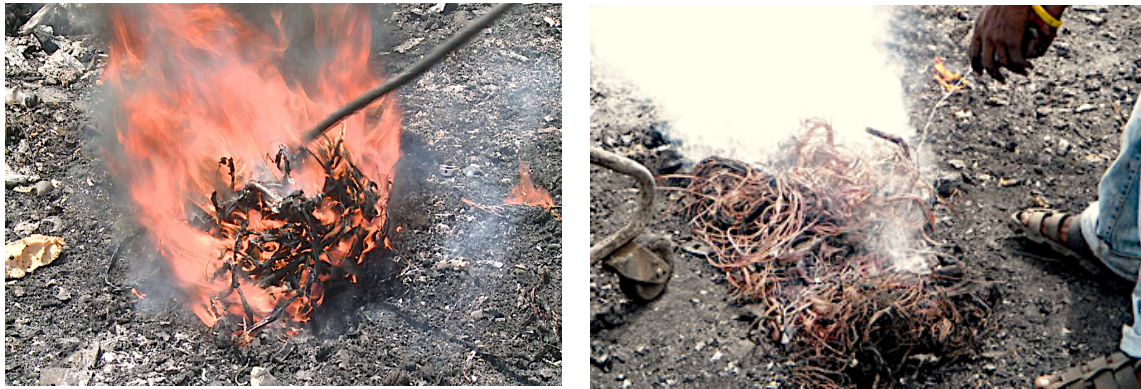
Photo 5. Burning and cooling of cables to retrieve copper scrap
