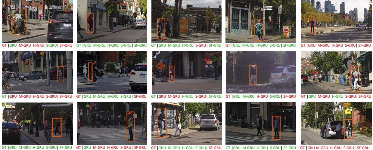
Figure 8.3: Examples of the predictions produced by the proposed algorithm SF-GRU and top competing methods, namely GRU , M-GRU , H-GRU , and S-GRU . In the examples, GT stands for ground truth and green and red colors indicate whether the pedestrian will cross in front of the ego-vehicle or not respectively. The instances where the color of the algorithm labels matches the GT means that their predictions are correct.
