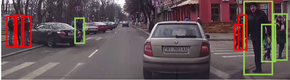
Figure 5.9: Selecting relevant objects in the scene with the aid of communication cues. Relevant and irrelevant pedestrians are shown with green and red boxes respectively.
