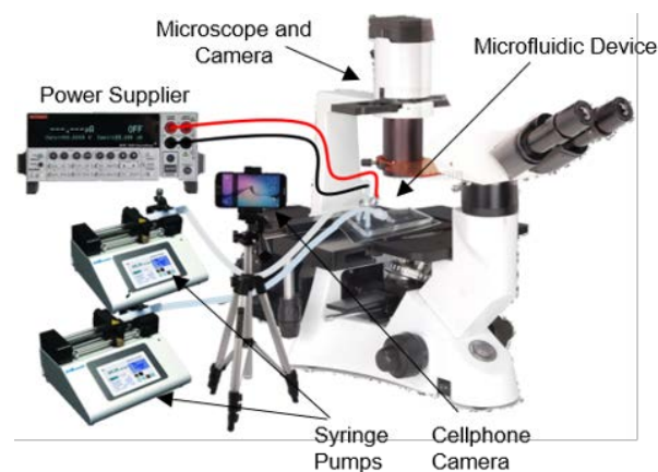
Figure 3-2. The experimental set-up consisted of the microfluidic device, two syringe pumps, direct current sourcemeter, microscope and two cameras, one on the microscope for close-up imaging and another on a stand for movement recording of the zebrafish larvae.
